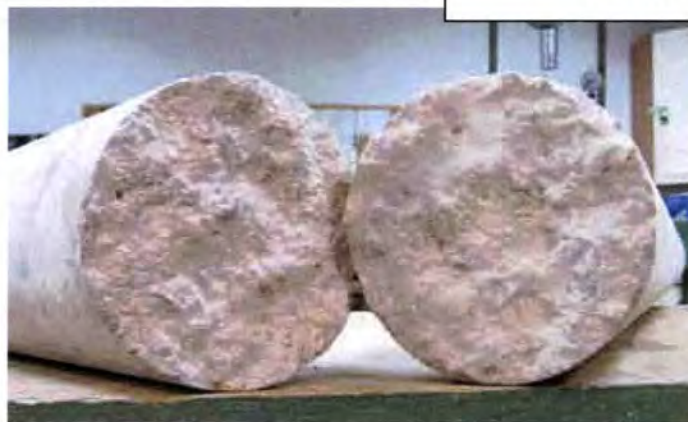
Photo 22: Core 4, Segments 6 and 7 - Cross section of break shows evidence of wearing.
