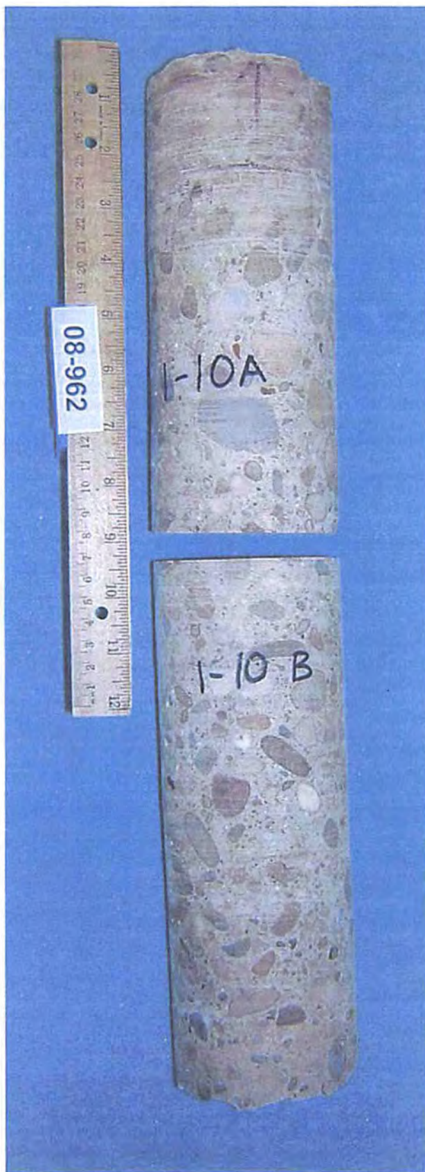
Photo 1. Side view of Core 1-10, received in two segments, identified as 1-10A and 1-10B, as received for testing.
