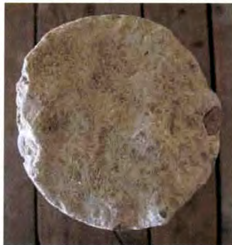
Photo 15: Core 3, Segment 7 - Evidence of wearing across joint.
