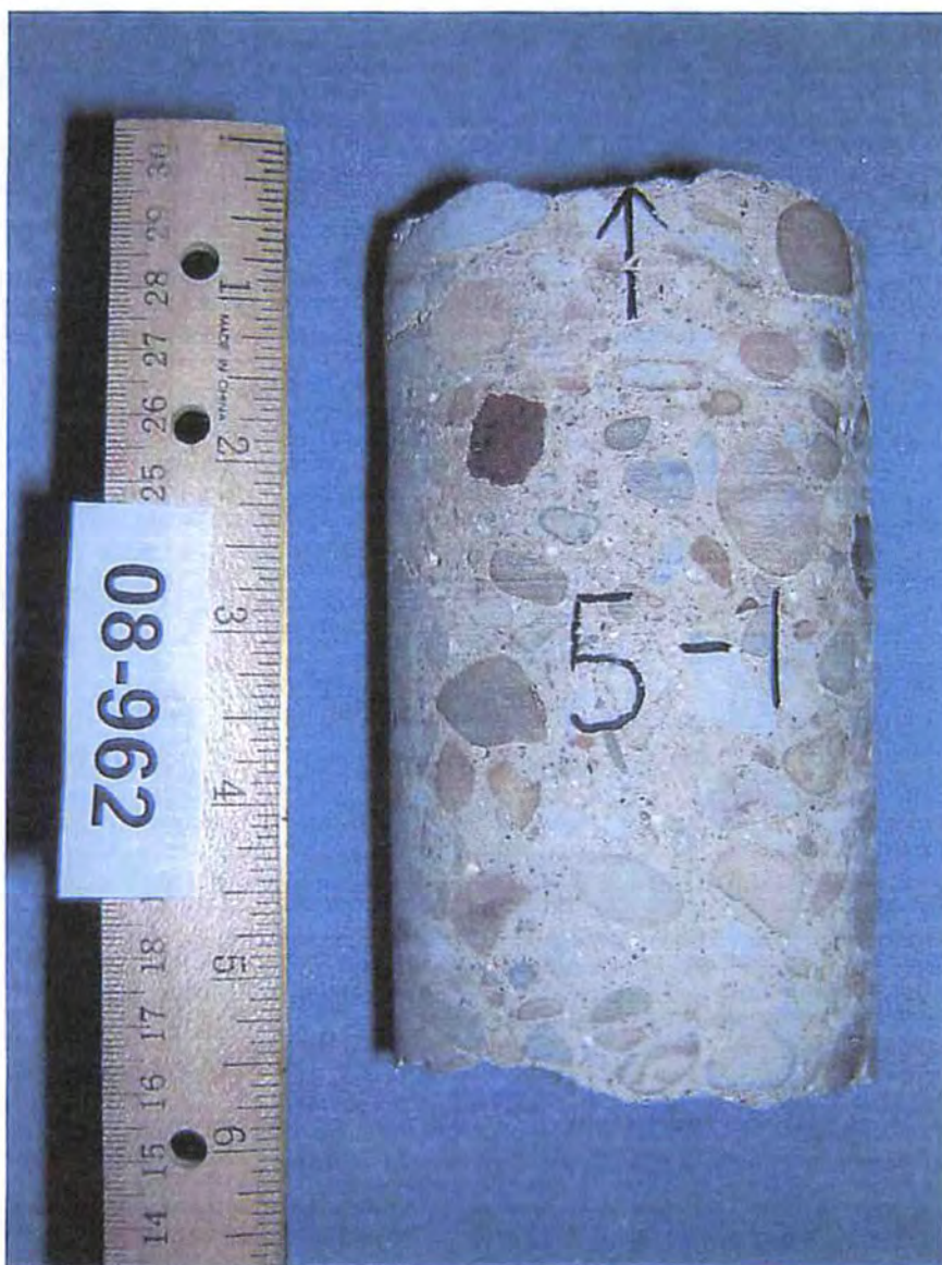
Photo 3. Side view of Core 5-1, as received for testing.
