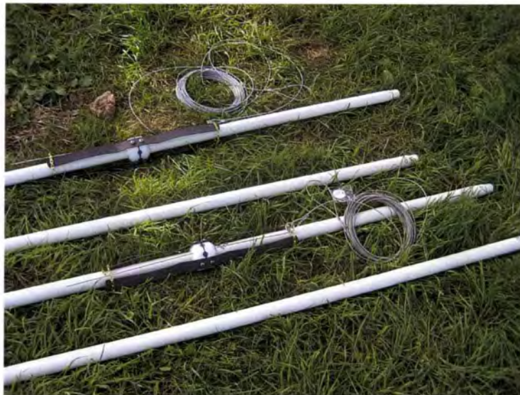
PHOTO 6: Extensometer measurement rings with pull cable, before installation
