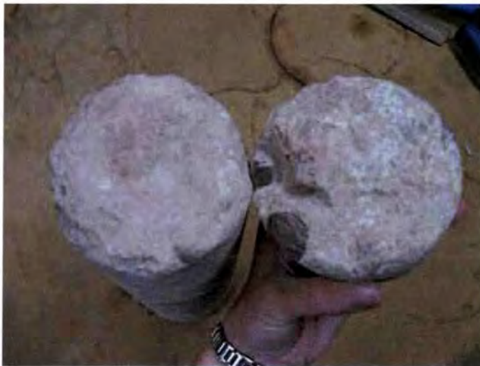
Photo 21: Core 4, Segments 4 and 5 - Cross section of break shows evidence of wearing.
