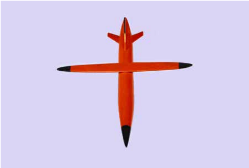
Proposed oblique-wing modification to a Teledyne-Ryan BQM-34F Firebee Drone, 1974. (NASA)
