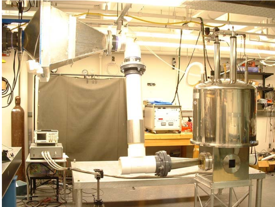
Facility with Mach 3 nozzle, superconducting magnet (6.5 T, 2.5-inch bore), and 30 kV, 100 kHz, 2 ns pulser
