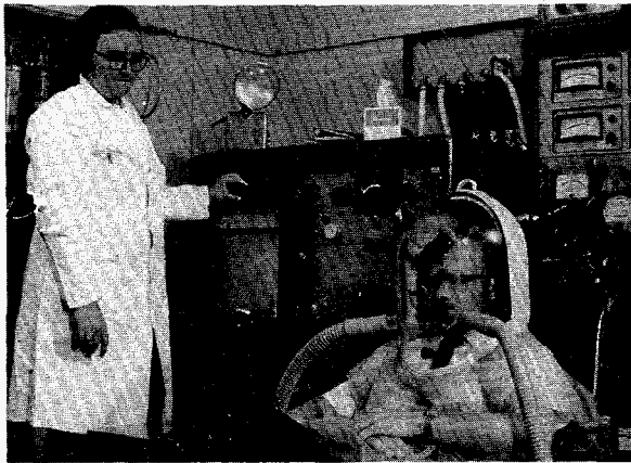
Figure 9. Donner Laboratory carbon-14 metabolic study apparatus.
