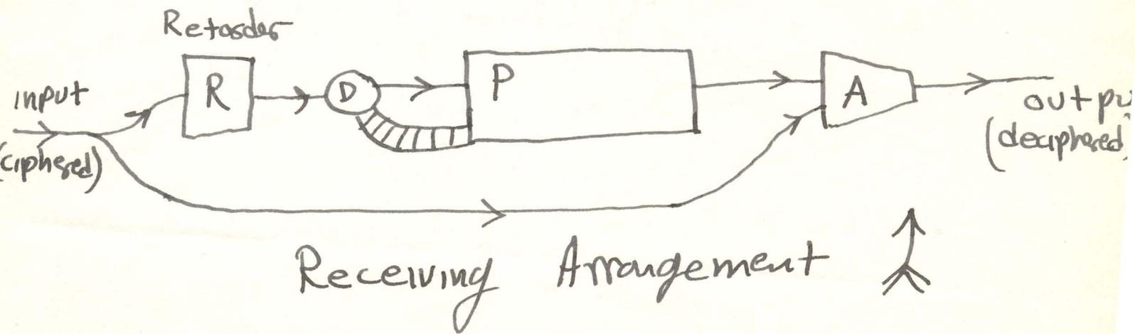
In the receiving arrangement the same components are used except for the addition of the retarder, which is a one-unit delay. The messages are to be sequences of binary digits (numbers mod 2). The machines work on a cycling basis, performing certain operations
