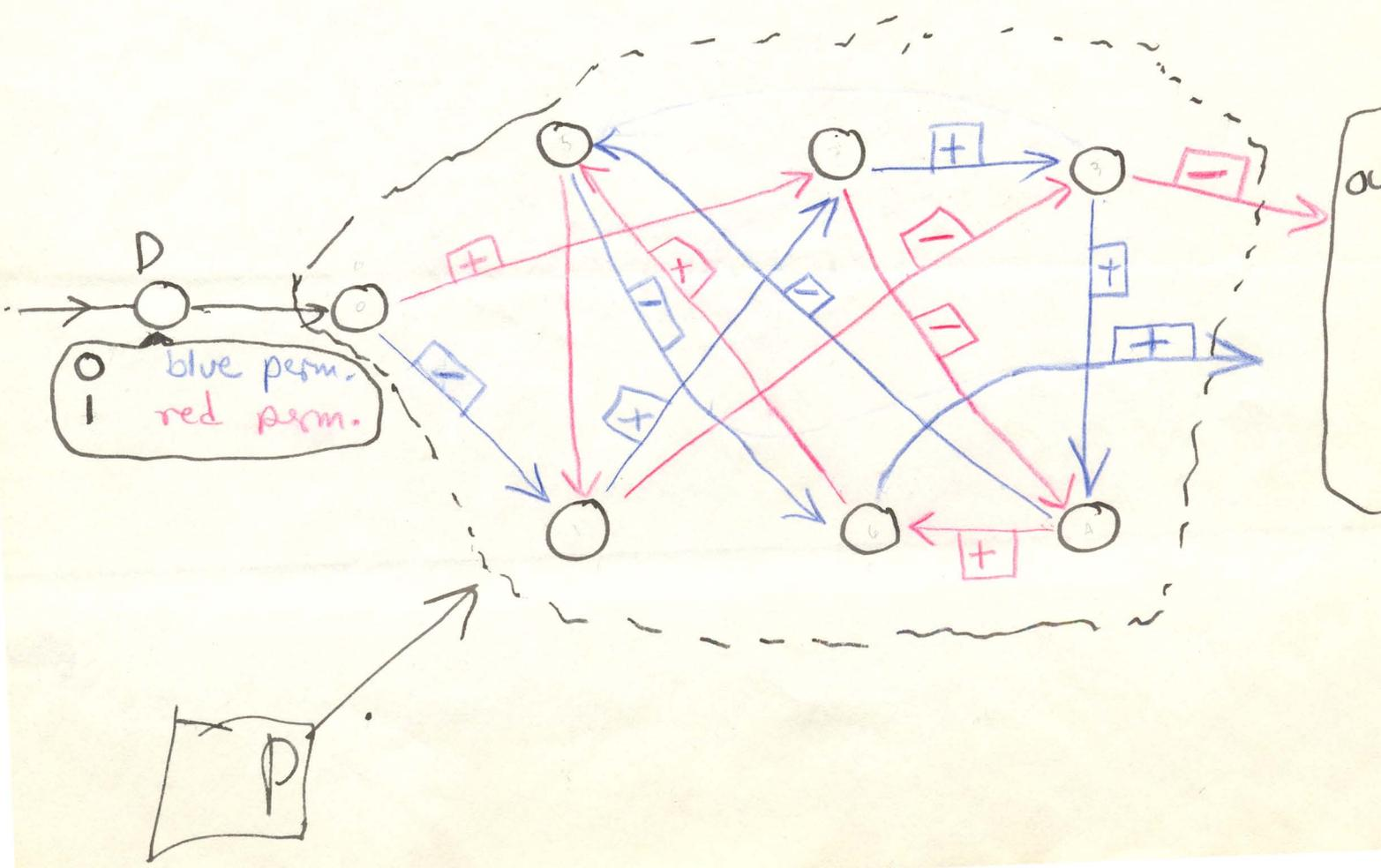
The circles represent places where a digit can be stored. During each cycle either the red permutation of digits or the blue takes place. This is decided by the digit in D at the beginning of the cycle. The D digit moves to the first circle or storage place in P during the cycle after it has determined the choice of the permutation.
