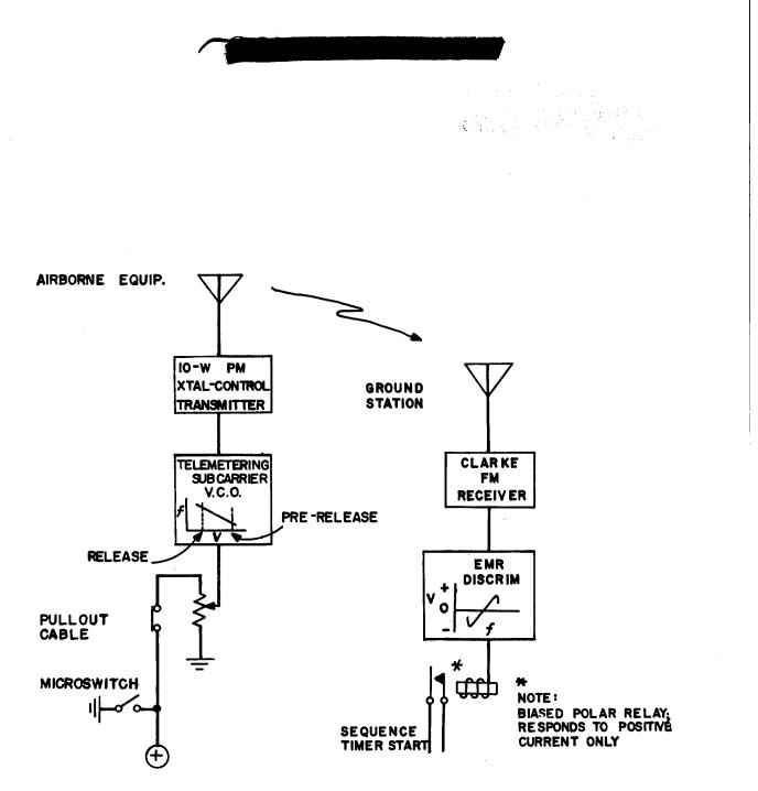
Fig. 4 -- Release Tone System, Basic Block Diagram
