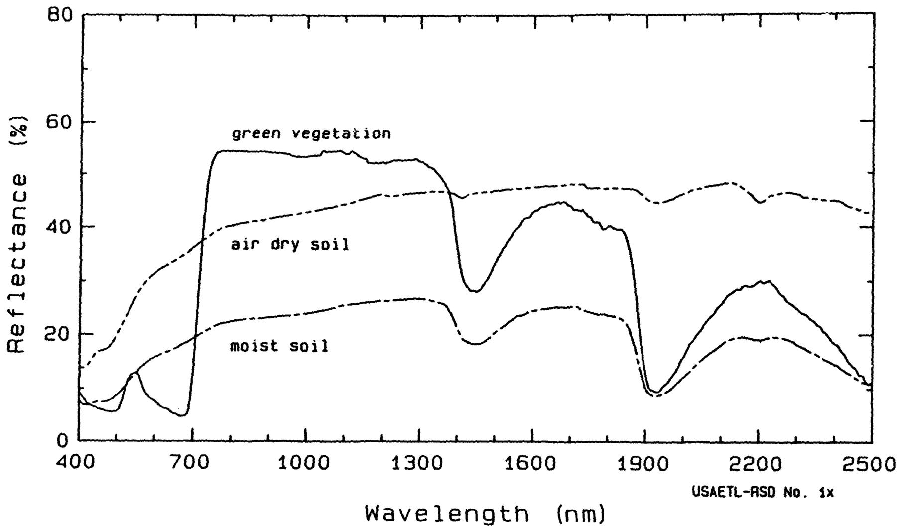
FIGURE B2. Air Dry and Moist Soil Surfaces and Green Vegetation.
