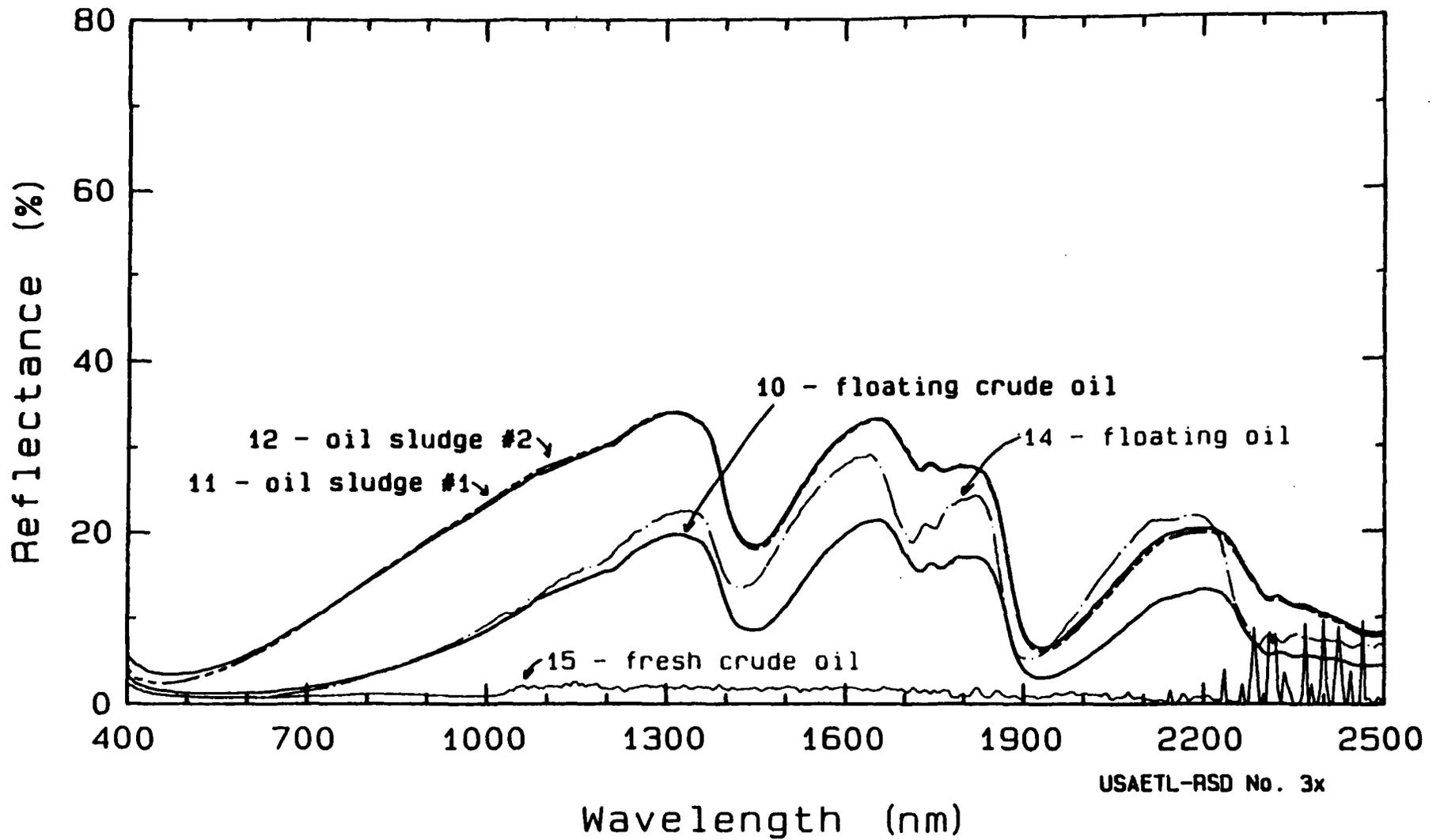
FIGURE B1. Spectra of Fresh and Weathered Oil
