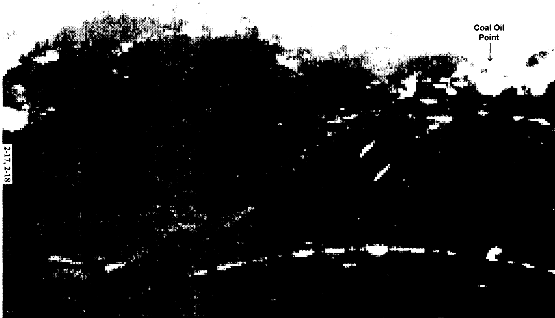
Figure 2-7. SLAR image of oil slick seen in Figure 2-5. Magnified by pixel replication. The contrast has been stretched to highlight the slick.
