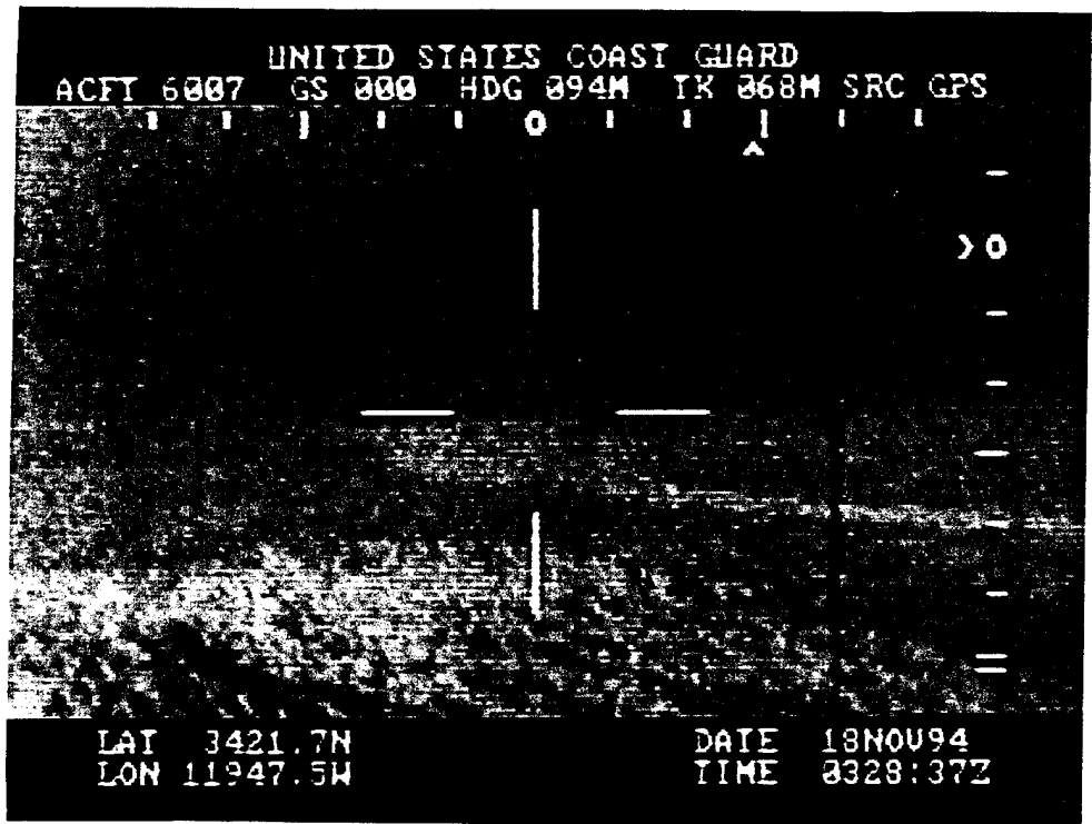
Figure 2-3. FLIR 2000 Image of the Area 3 Slick, 17 November 1994 (Black = Hot, Narrow Field of View)
