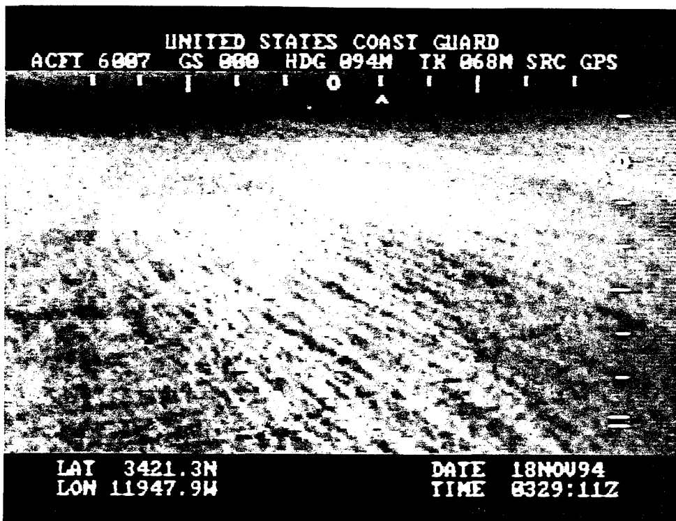
Figure 2-2. FLIR 2000 Image of the Area 3 Slick, 17 November 1994 (Black = Hot, Wide Field of View)
