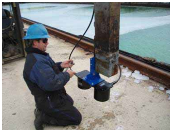
Figure 24. BioSonics DT-X Digital Scientific Echosounder sensor.
