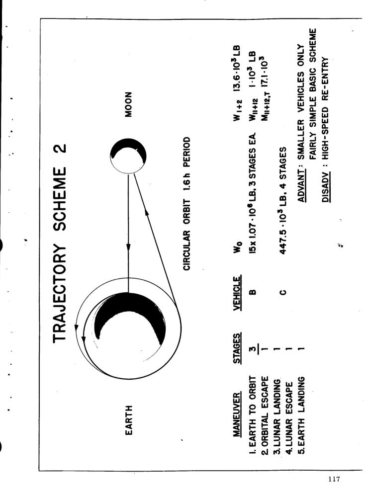
So from fifteen such flights, we build together a unit of this size, which can do the whole trick, in lieu of having one like the single earth-based one.
