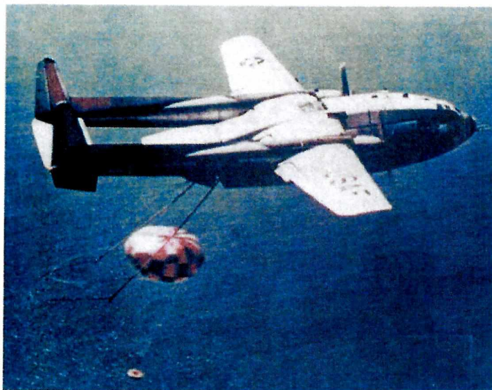
Figure 7. Successful mid-air recovery by a C-119J Flying Boxcar
