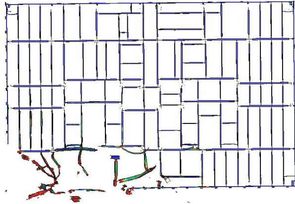
(b) Floor 81 core framing damage
