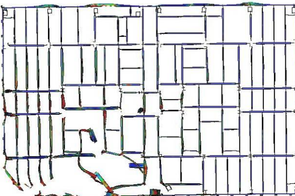
(c) Floor 80 core framing damage
