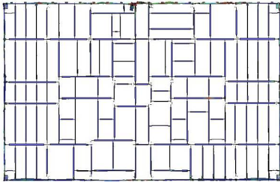
(a) Floor 93 core framing damage
