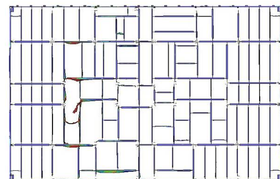
(f) Floor 98 core framing damage
