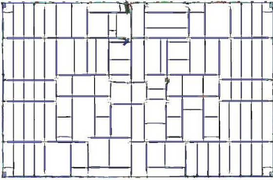
(a) Floor 93 core framing damage
