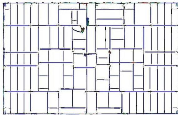
(a) Floor 93 core framing damage
