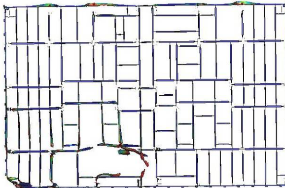
(c) Floor 79 core framing damage
