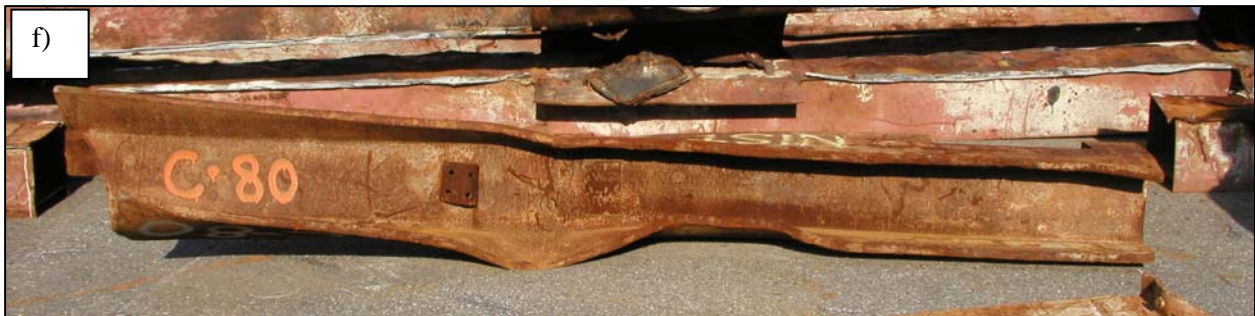
Figure 3–12. Core columns recovered from WTC 1. e) C-71 (904A: 77–80), lower 16 ft of wide flange section, f) C-80 (603A: 92–95), lower 13 ft of wide flange section (continued).
