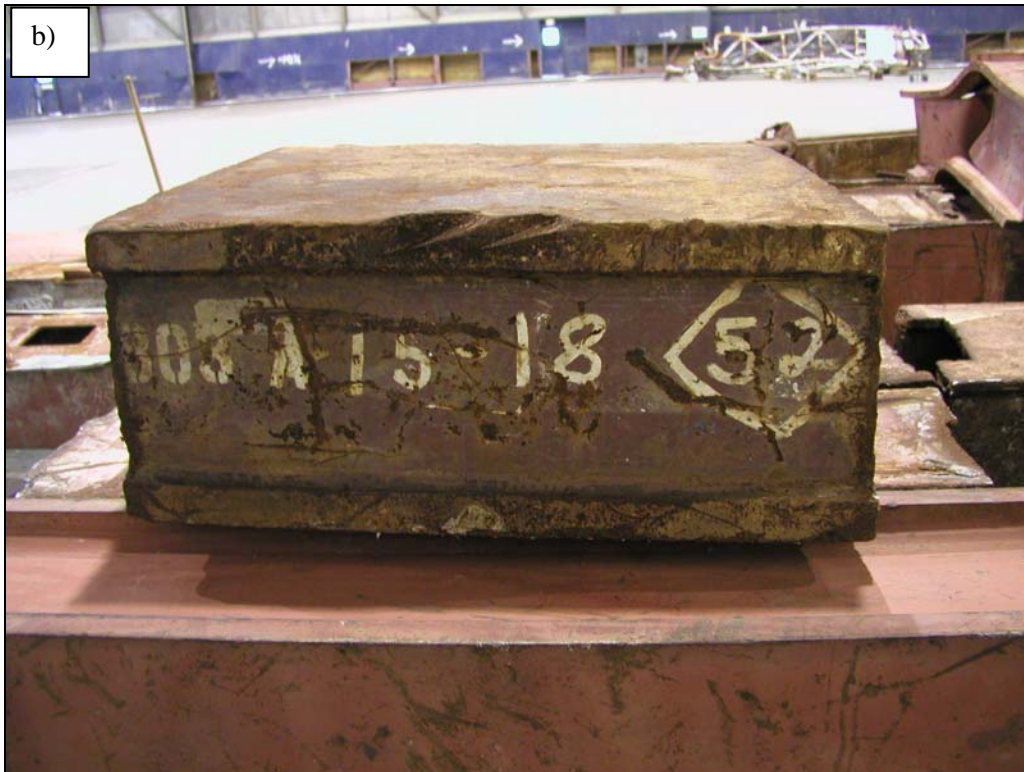
Figure 3–12. Core columns recovered from WTC 1. a) B-1011 (508A: 51–54), lower 2 ft to 3 ft of built-up box column, b) B-6152-1 (803A: 15–18), lower 3 ft of built-up box column.
