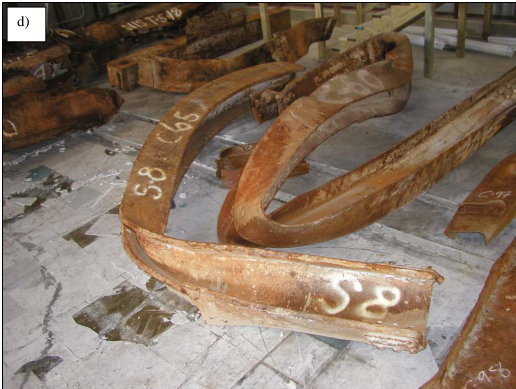
Figure 3–12. Core columns recovered from WTC 1. c) B-6152-2 (504A: 33–36), lower 2 ft of built-up box column, d) C-65 (904A: 86–89), lower 24 ft of wide flange section (continued).
