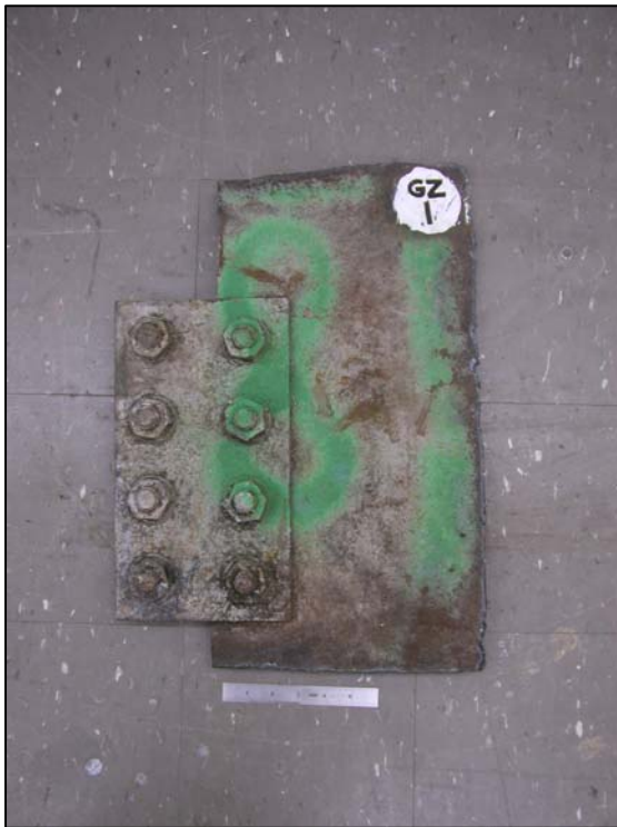
Figure A-12. Coupons removed in the field from WTC 5; shown is sample GZ-1.
