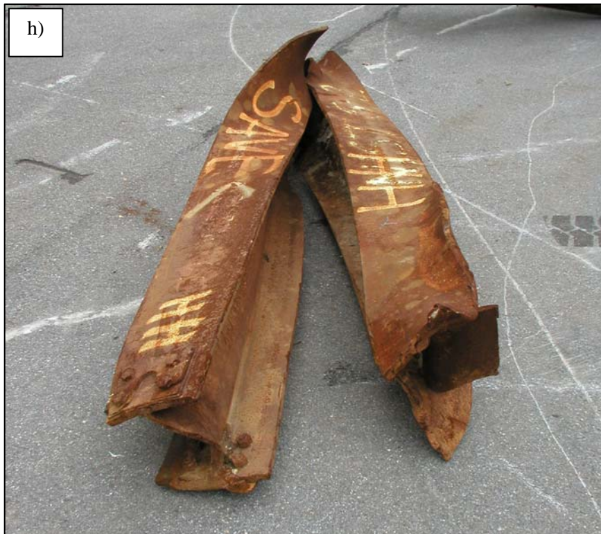
Figure 3–12. Core columns recovered from WTC 1. g) C-155 (904A: 83–86), lower 33 ft of wide flange section, and h) HH (605A: 98–101), lower 16 ft of wide flange section (continued).
