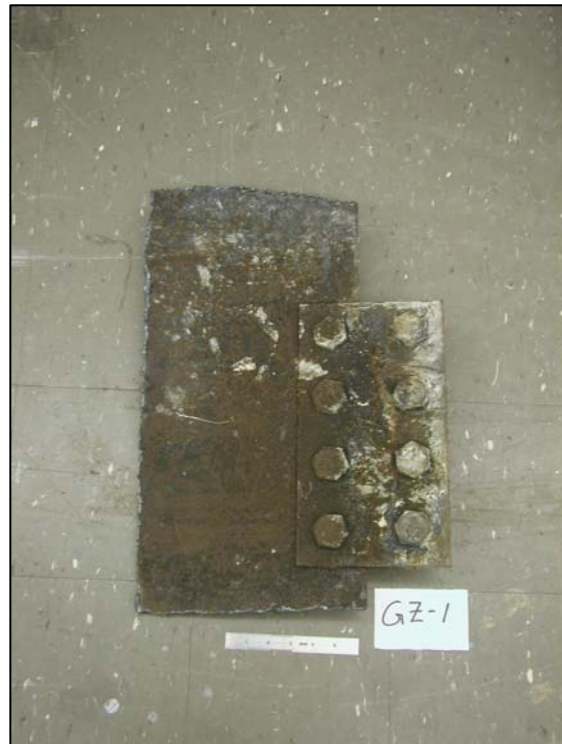
Figure A-12. Coupons removed in the field from WTC 5; shown is sample GZ-1.
