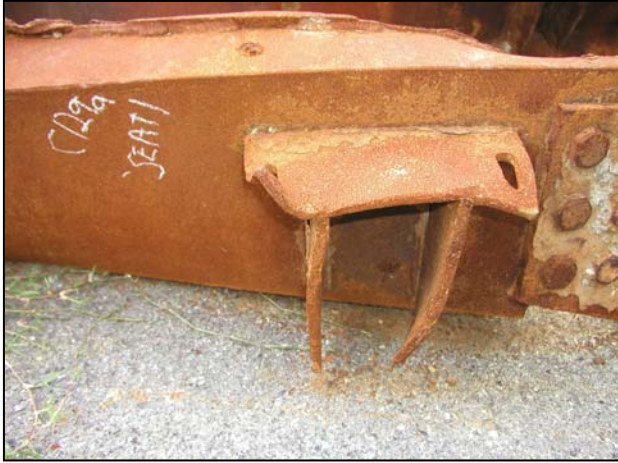
Seat 1a: One hole intact, other ripped out, seat was bent
