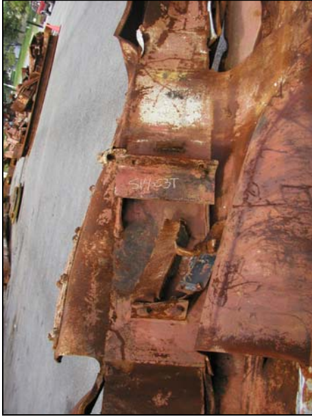
S14-C3M (WTC 2, Col.217, Fl 93) Type A Seat Detail: 1611
