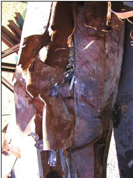
Figure B-38. Floor truss connectors found on recovered panel S-9 (A133: 97-100) from WTC 1. Shown are connectors found on column 133 at different floor levels (cont.).
