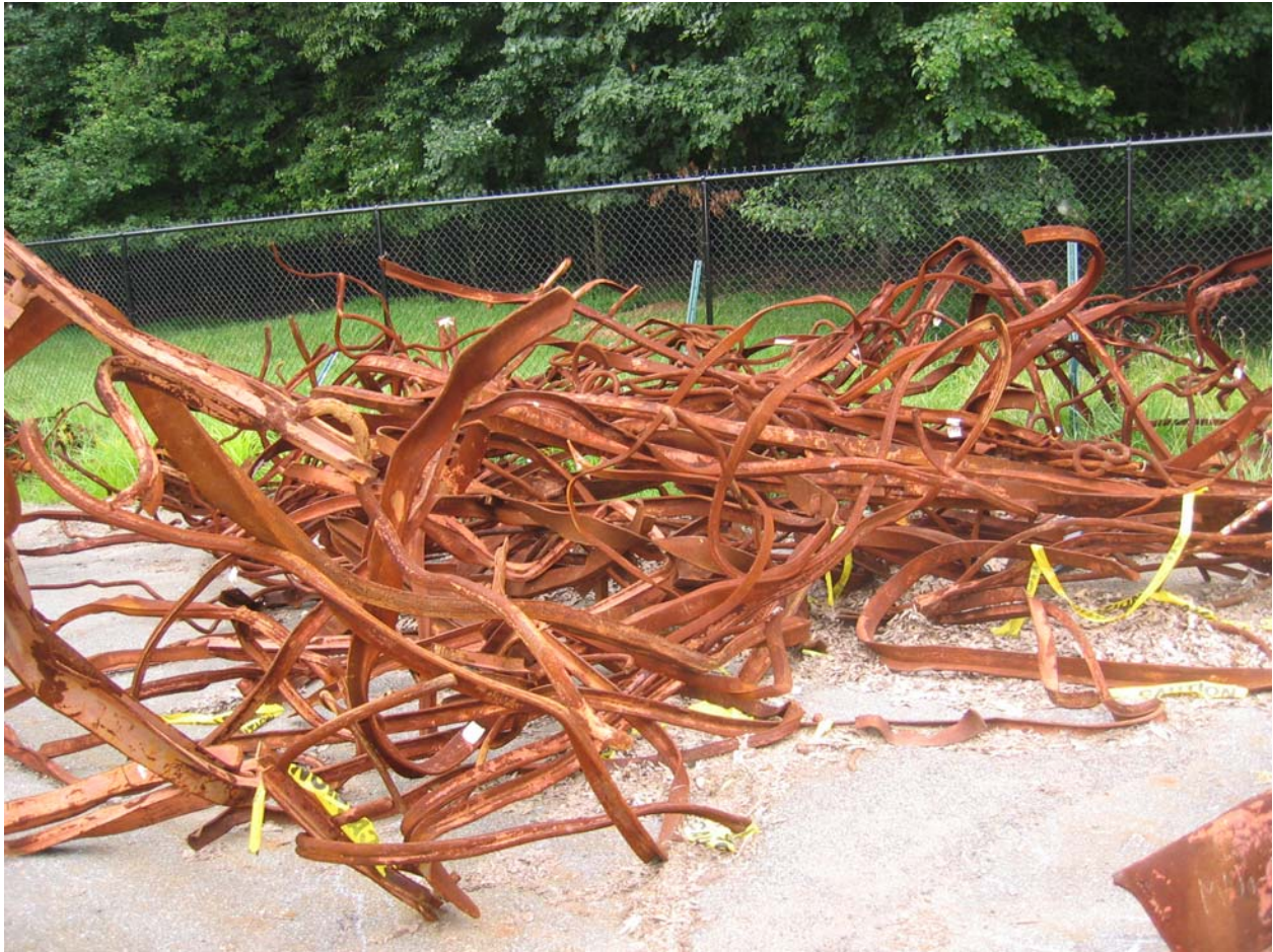
Figure 18. General view of a portion of recovered floor truss material
