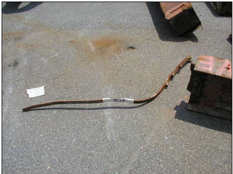
Figure A3b: Type C floor truss connector
