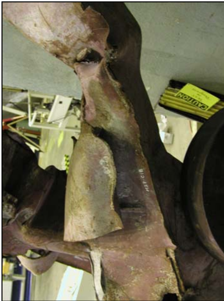
Figure B-25. Floor truss connectors found on recovered panel M-27 (A130: 93-96) from WTC 1. Shown are connectors found on column 131 at different floor levels.
