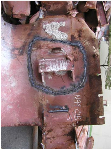
Figure B-35. Floor truss connectors found on recovered panel N-99 (A148: 99-102) from WTC 1. Shown are connectors found on column 149 at different floor levels.
