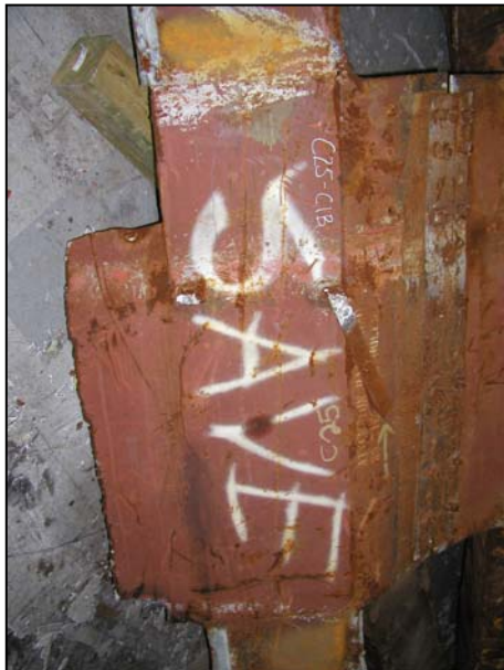
Figure B-8. Floor truss connectors found on recovered panel C-25 (A206: 89-92) from WTC 1. Shown are connectors found on column 207 at different floor levels.
