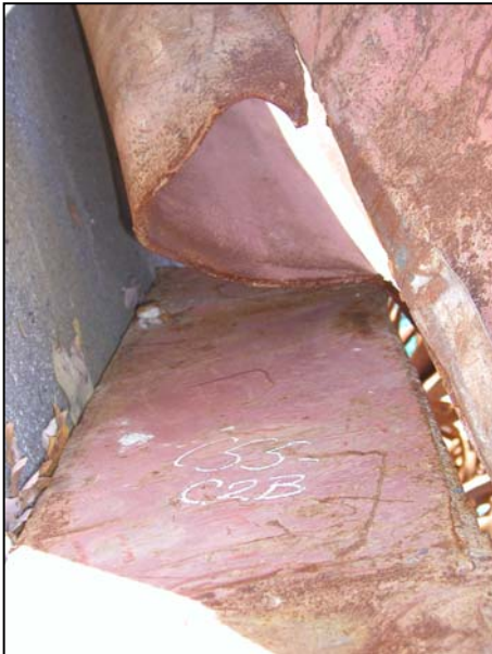
Figure B-12. Floor truss connectors found on recovered panel C-55 (A209: 94-97) from WTC 1. Shown are connectors found on column 209 at different floor levels (cont.).
