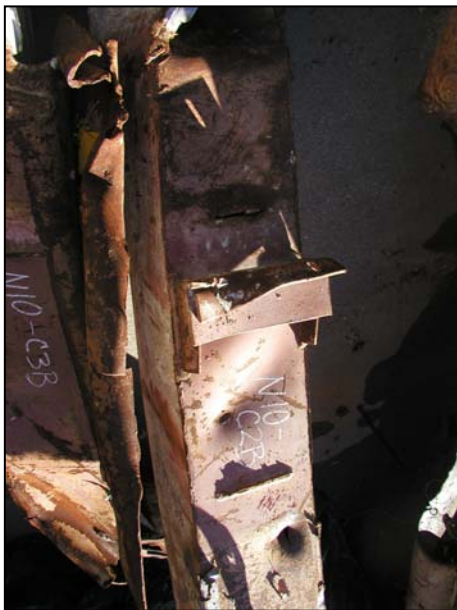
Figure B-32. Floor truss connectors found on recovered panel N-10 (A115: 89-92) from WTC 1. Shown are connectors found on column 115 at different floor levels (cont.).
