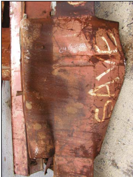
Figure B-11. Floor truss connectors found on recovered panel C-48 (B442: 91-94) from WTC 2. Shown are connectors found on column 442 at different floor levels (cont.).
