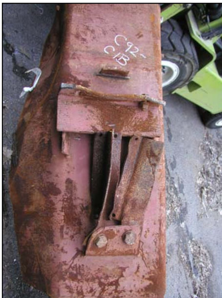
Figure B-14. Floor truss connectors found on recovered panel C-92 (B130: 93-96) from WTC 2. Shown are connectors found on column 131 at different floor levels.
