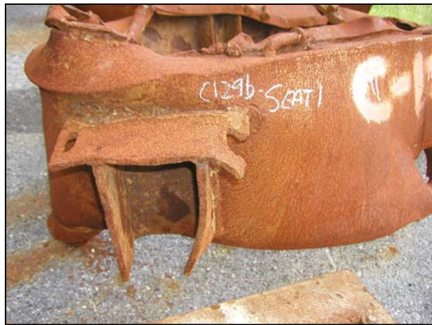
Seat 1a: One hole intact, other ripped out, seat was bent
