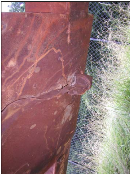
Figure B-13. Floor truss connectors found on recovered panel C-89 (B215: 12-15) from WTC 2. Shown are connectors found on column 215 at different floor levels (cont.).
