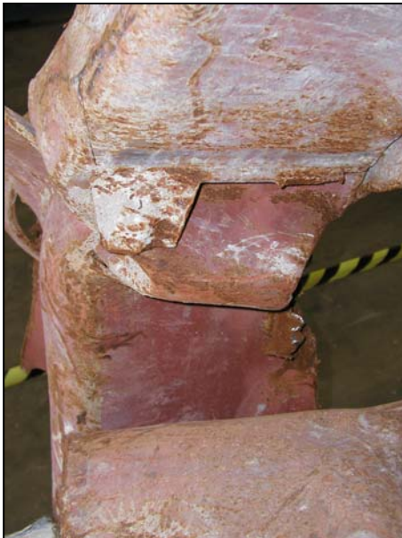
Figure B-25. Floor truss connectors found on recovered panel M-27 (A130: 93-96) from WTC 1. Shown are connectors found on column 130 at different floor levels (cont.).
