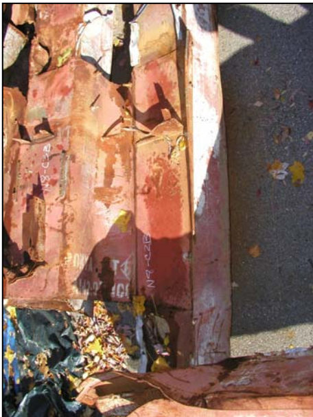
Figure B-30. Floor truss connectors found on recovered panel N-8 (A142: 97-100) from WTC 1. Shown are connectors found on column 142 at different floor levels (cont.).
