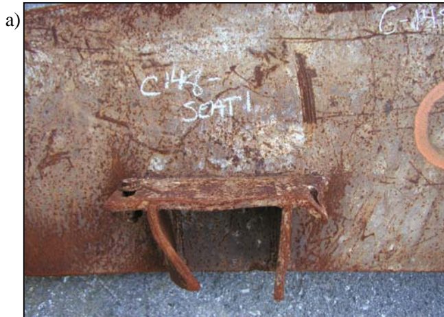
Seat 1: Both holes intact, one has bolt
