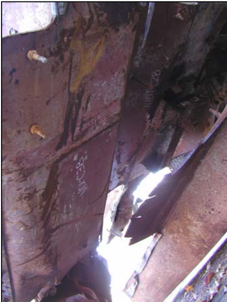
Figure B-36. Floor truss connectors found on recovered panel N-101 (A133: 100-103) from WTC 1. Shown are connectors found on column 132 at different floor levels (cont.).
