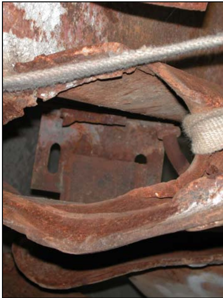
Figure B-4. Floor truss connectors found on recovered panel C-14 (B300: 85-87) from WTC 2. Shown are connectors found on column 259 at different floor levels (cont.).
