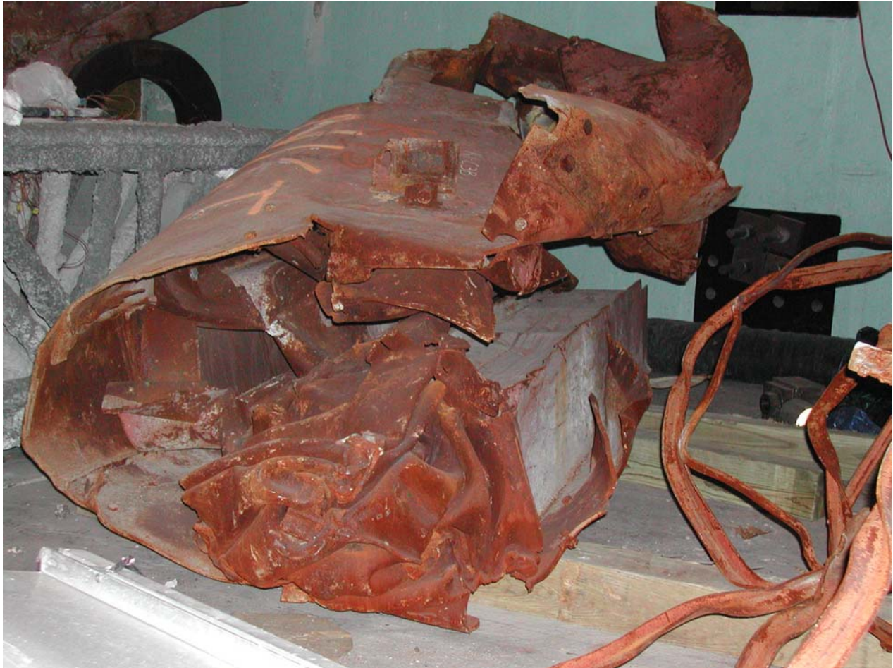
Figure 22. Piece K-1, which has collapsed in compression
