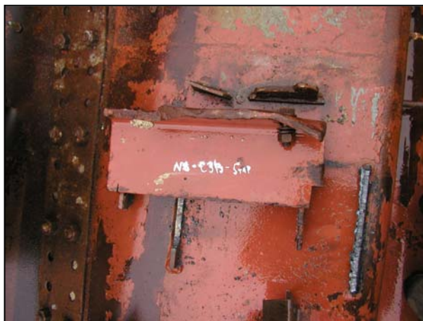
Figure B-30. Floor truss connectors found on recovered panel N-8 (A142: 97-100) from WTC 1. Shown are connectors found on column 141 at different floor levels subsequent to their removal for mechanical property testing (cont.).
