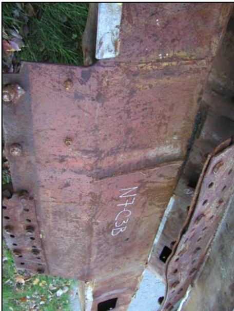
Figure B-29. Floor truss connectors found on recovered panel N-7 (A127: 97-100) from WTC 1. Shown are connectors found on column 126 at different floor levels (cont.).
