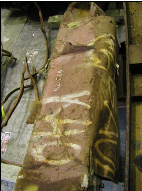
Figure B-19. Floor truss connectors found on recovered panel K-2 (A236: 92-95) from WTC 1. Shown are connectors found on column 236 at different floor levels (cont.).
