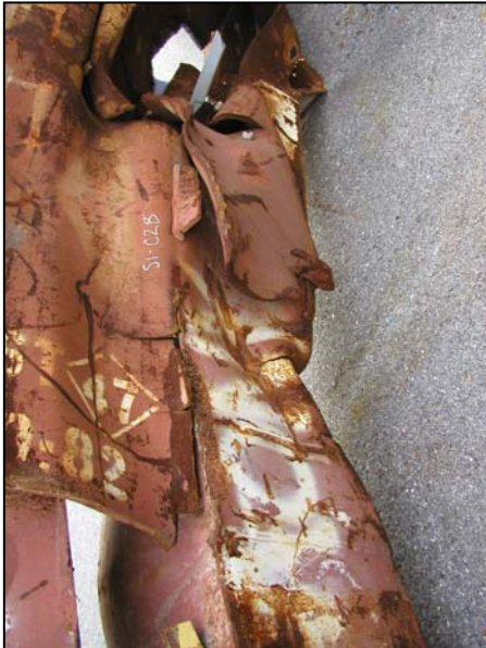
Figure B-37. Floor truss connectors found on recovered panel S-1 (A433: 79-82) from WTC 1. Shown are connectors found on column 433 at different floor levels (cont.).
