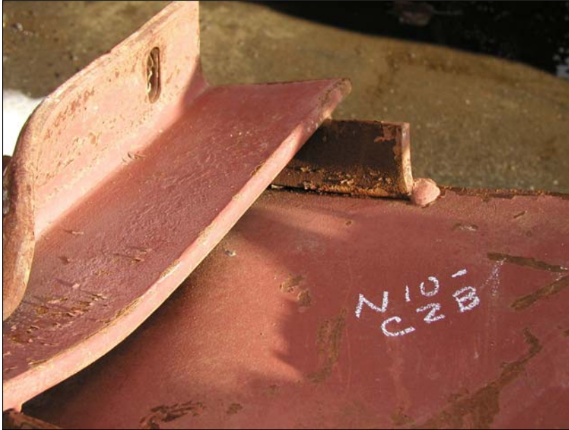
Figure A1c: Type A floor truss connector
