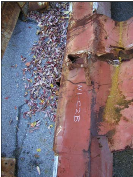
Figure B-28. Floor truss connectors found on recovered panel N-1 (A218: 82-85) from WTC 1. Shown are connectors found on column 218 at different floor levels (cont.).
