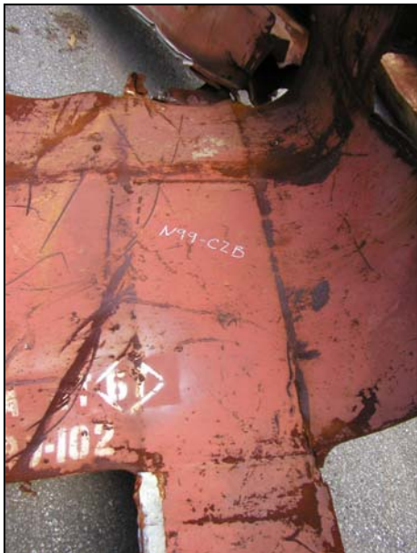
Figure B-35. Floor truss connectors found on recovered panel N-99 (A148: 99-102) from WTC 1. Shown are connectors found on column 148 at different floor levels (cont.).
