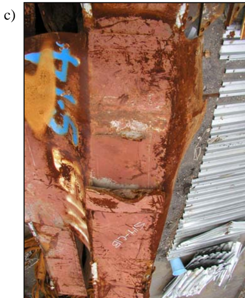
Figure B-40. Floor truss connectors found on recovered panel S-14 (B218: 91-94) from WTC 2. Shown are connectors found on column 219 at different floor levels.
