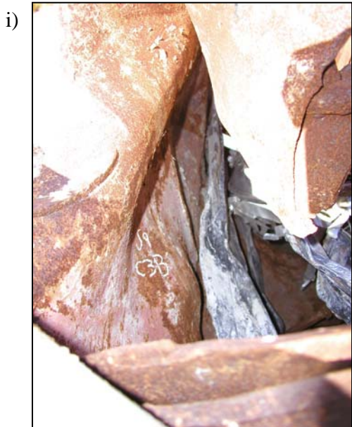
Figure B-38. Floor truss connectors found on recovered panel S-9 (A133: 97-100) from WTC 1. Shown are connectors found on column 132 at different floor levels (cont.).
