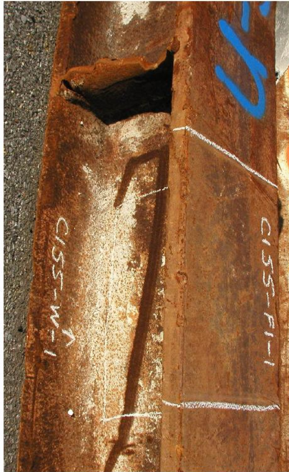
Figure B-6. Montage of specimen C-155 that shows the overall state of the column and the region that provided the test specimens.
