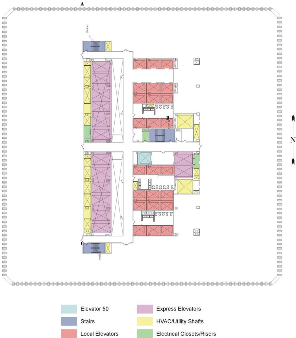
**Figure 5–3. Floor layout, 80th Floor, WTC 2, South Tower.**
