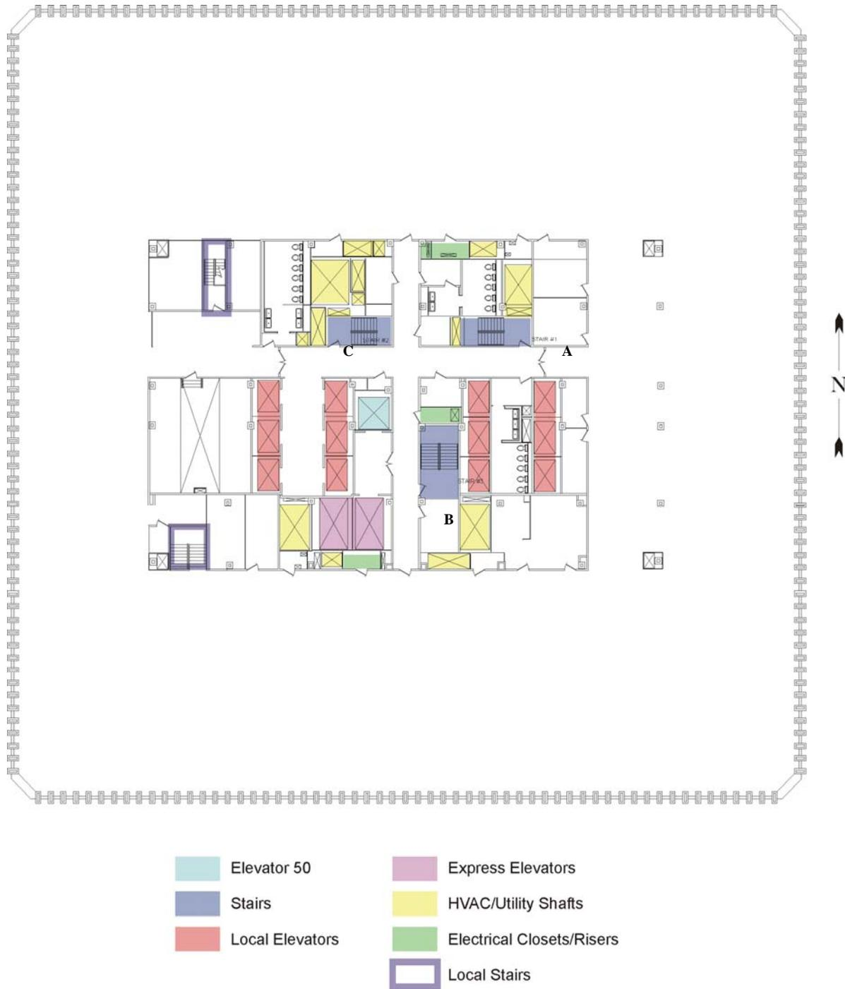
Figure 5–2. Floor layout, 95th floor, WTC 1, North Tower.
