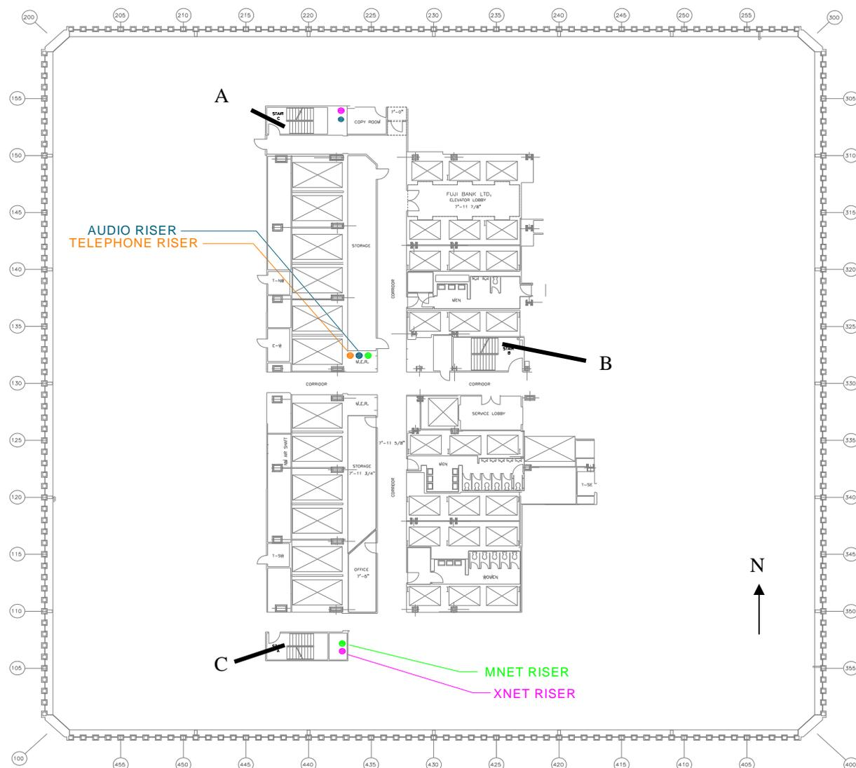
Figure 4–9. Typical WTC 2 riser locations on impact floors.
