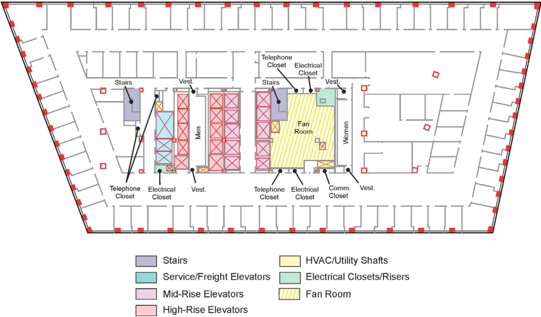
Figure 5-5. Floor layout, 24th floor, WTC 7.
