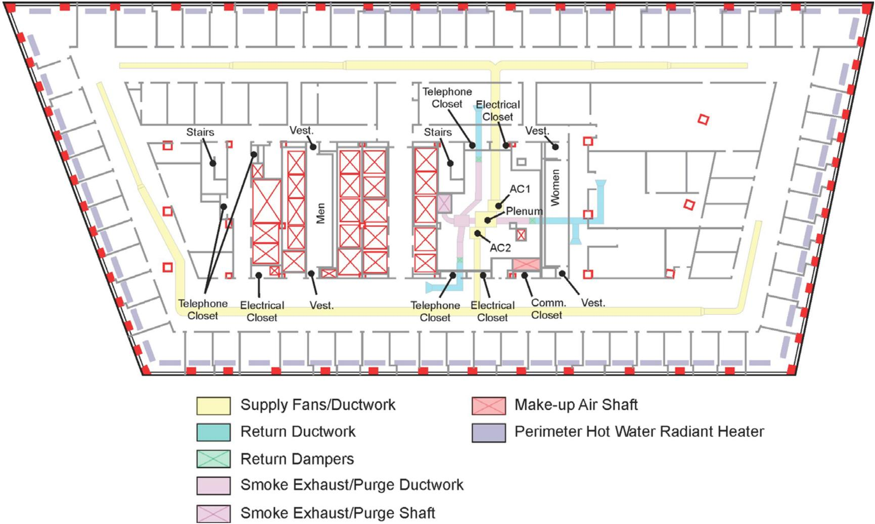
Figure 5-6. Air distribution system, 24th floor, WTC 7.
