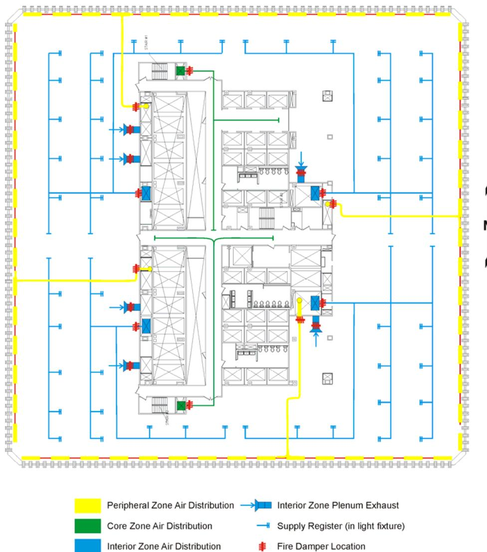
**Figure 5-7. Air distribution system, 80th floor, WTC 2.**
