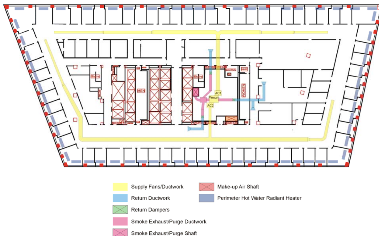
Figure 4–11. Air distribution system, 24th floor, WTC 7.
