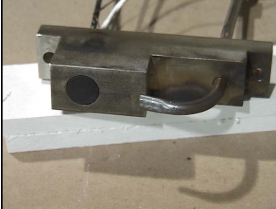
Figure 5–1. Flux gauge holder showing gauge sensor surface (black disc) and soot purge tube. Surface of gauge holder and gauge sensor surface were set flush with the surrounding Marinite cover on any monitored surface.
