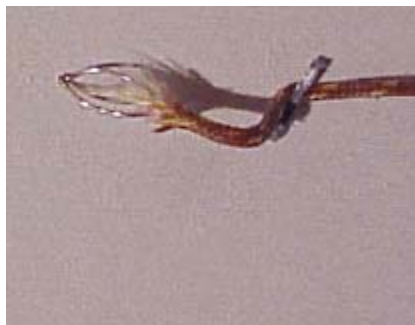
Figure 8–1. A type K thermocouple attached to the Marinite surface.
