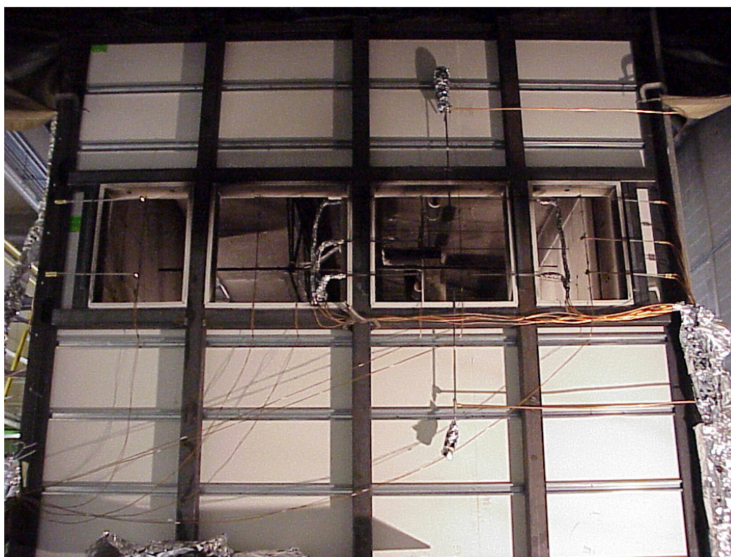
Figure 2–6. Instrumentation on the outside of the west wall of the compartment.
