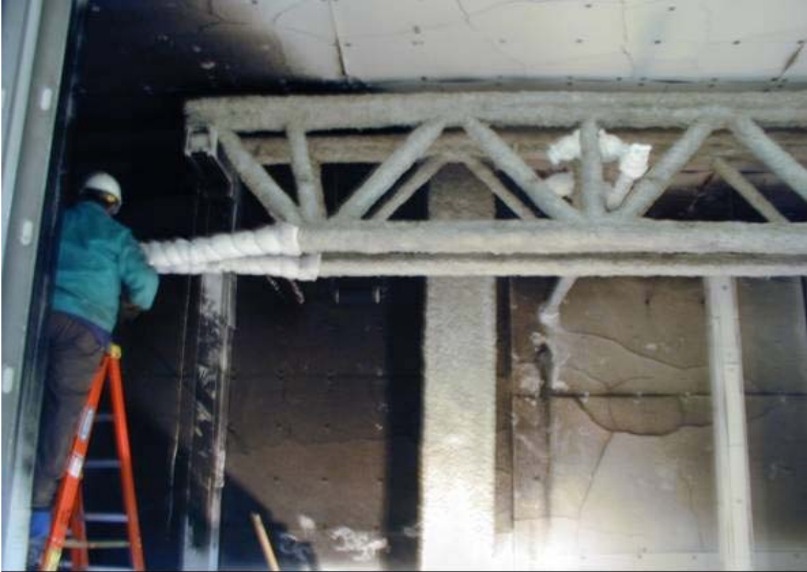
Figure 9–7d. Insulated steel components in test compartment for Tests 5 and 6.
