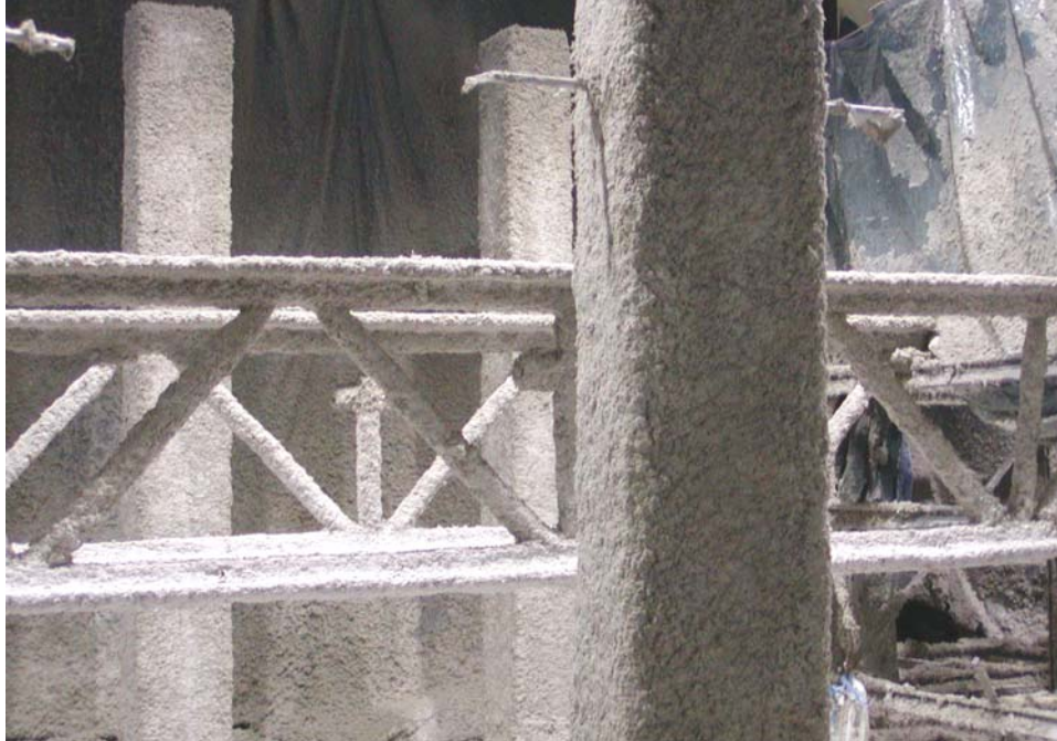
Figure 9-6e. Steel components with SFRM product prior to testing.
