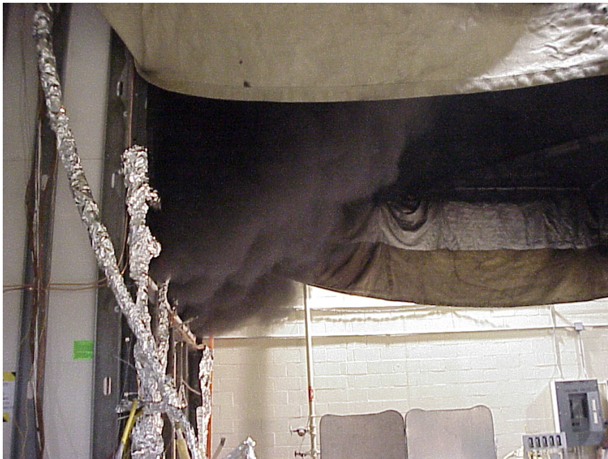
Figure 2–8. Smoke exiting the outlet vent into the exhaust hood during Test 2.
