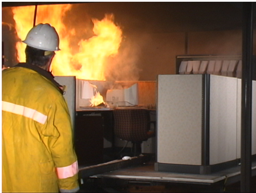
Figure 3–7b. First ignited object within cubicle, paper stack on desk, at approximately 60 s after start of 2 MW igniter flame.
