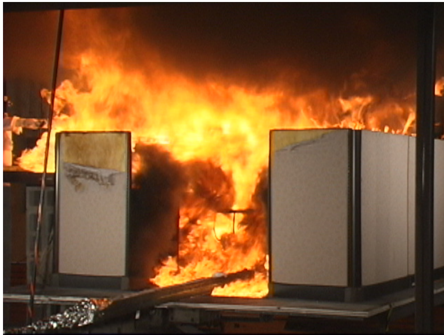
Figure 3–7e. Work station fire near peak HRR at 533 s.
