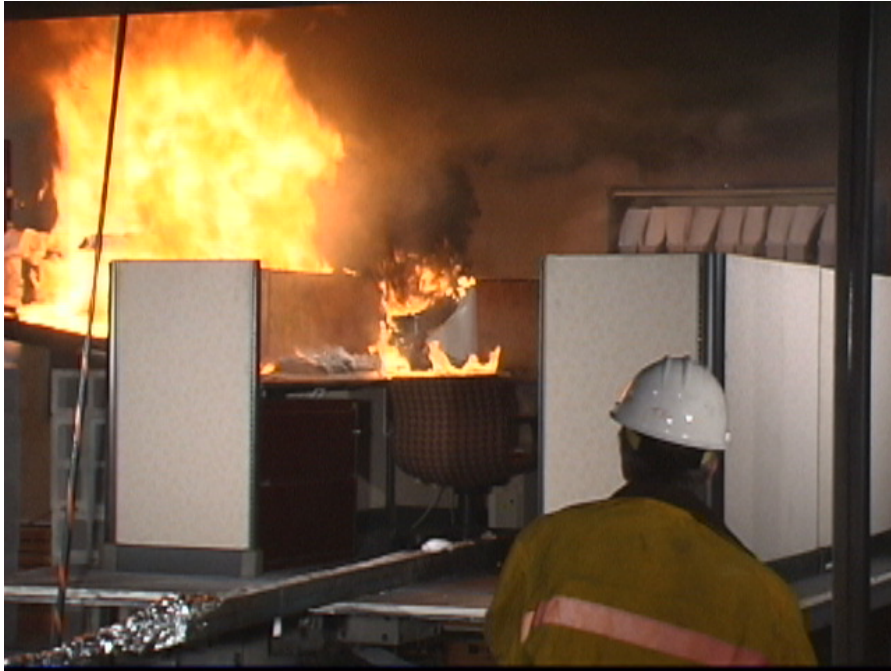
Figure 3–7c. Top of chair back ignited at about 165 s; computer already burning.
