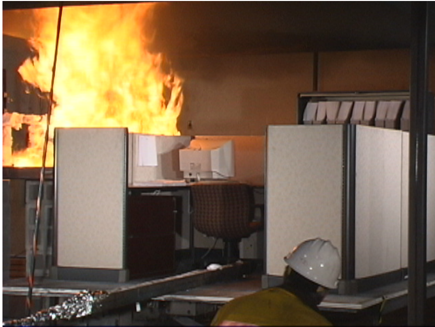
Figure 3–7a. 2 MW igniter flame at time zero.
