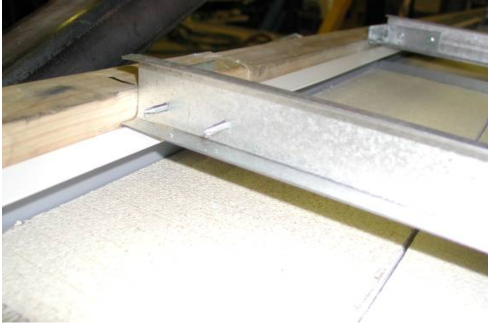
Figure 2–20. Channel section runner connection to edge of test frame in suspension system 1.
