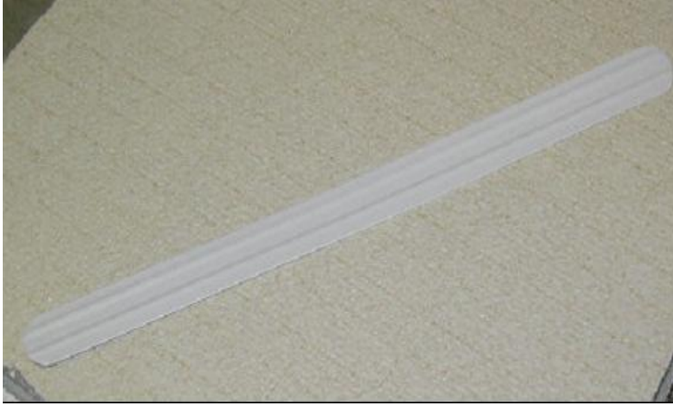
Figure 2–22. Breather spline used in suspension system 1.
