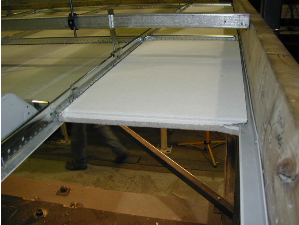
Figure 3–15. Damage to south perimeter of ceiling system CS4 after 1.75g earthquake excitation.
