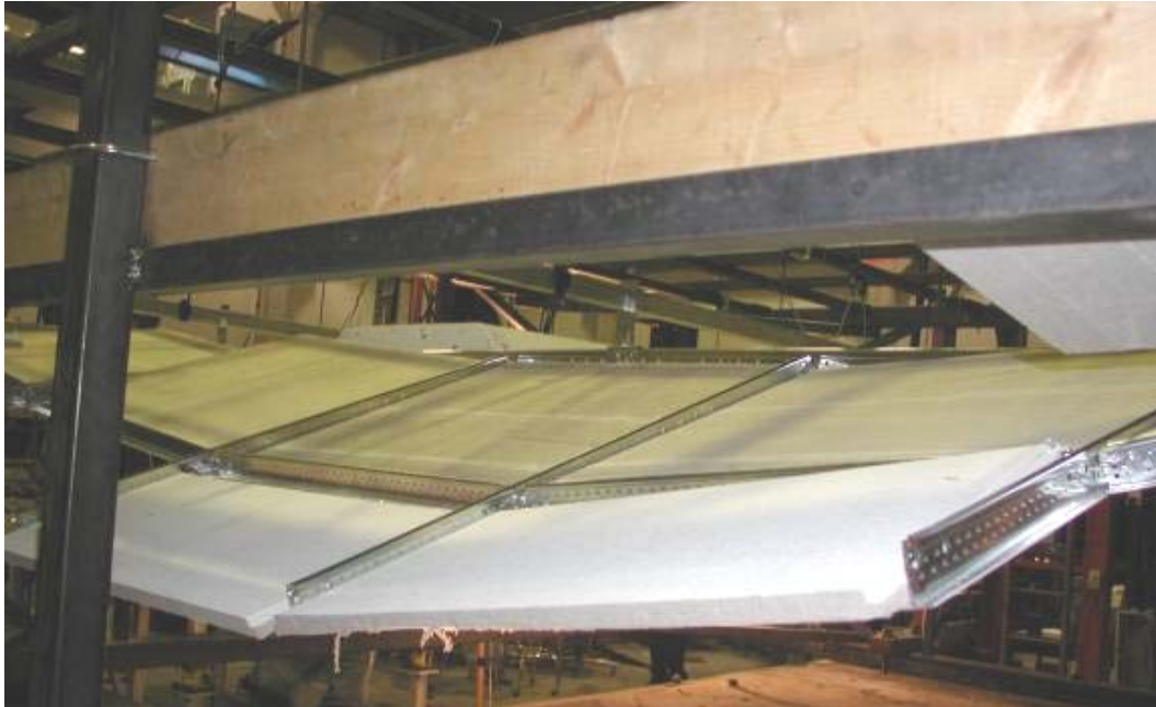
Figure 3–12. Damage to the northern perimeter of ceiling system CS4 following Test 23.
