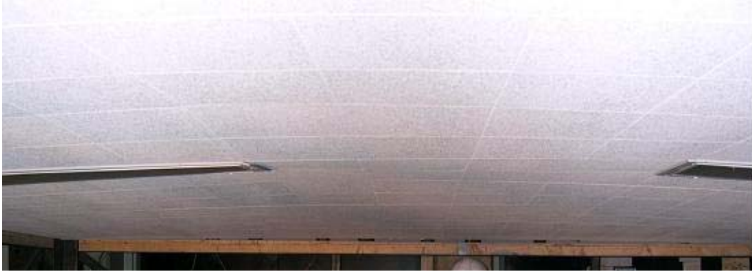
Figure 3–3. Bottom view of damage to ceiling system CS1 following Test 20.
