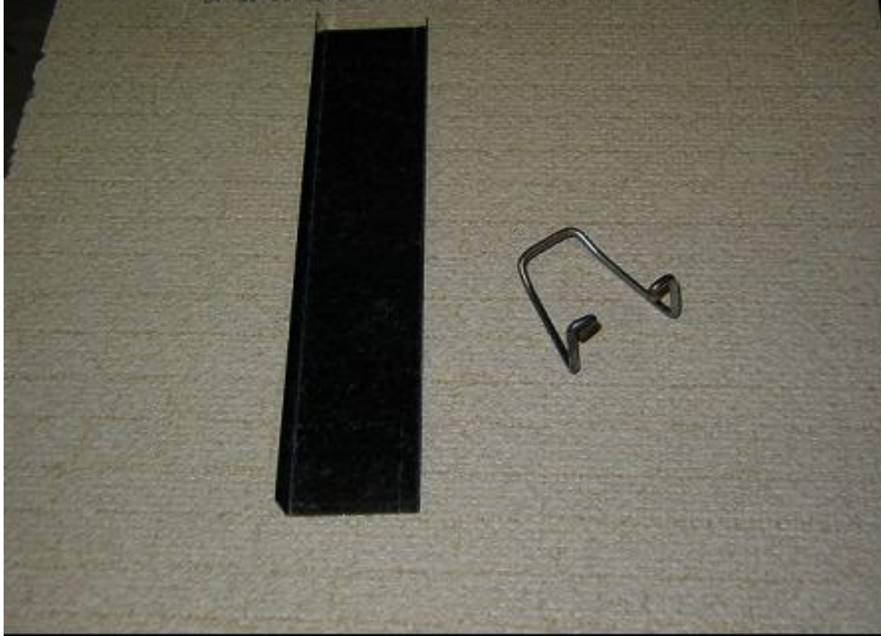
Figure 2–18. Z-bar section (left) and C-15 wire clip (right) in suspension system 1.
