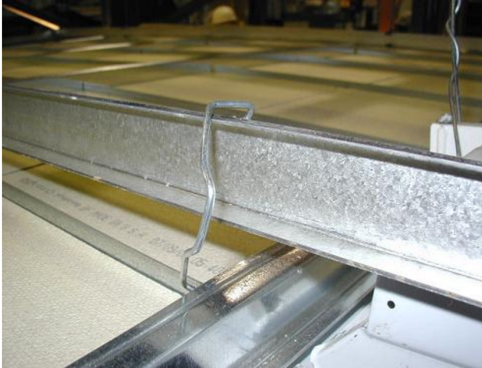
Figure 3–8. Stretching of Z-bar clips located at northern light fixture corner in ceiling system CS3 following Test 20.
