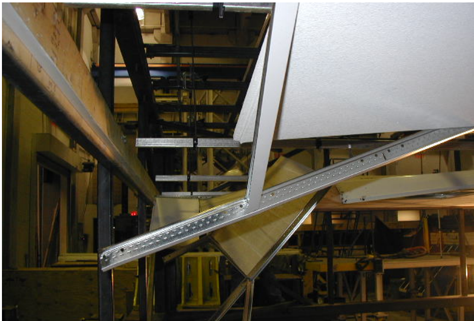
Figure 3–14. Damage to north perimeter of ceiling system CS4 after 1.75g earthquake excitation.
