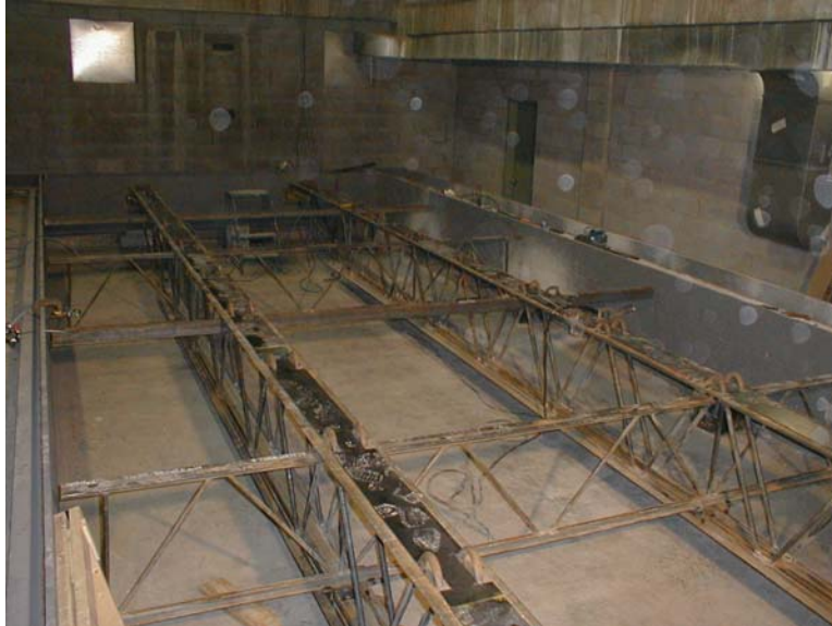
Figure 3–4. Trusses being fit-up in test frame of 35 ft test assembly.
