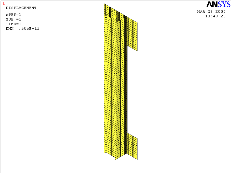
Figure 4-34. One-story exterior column model.
