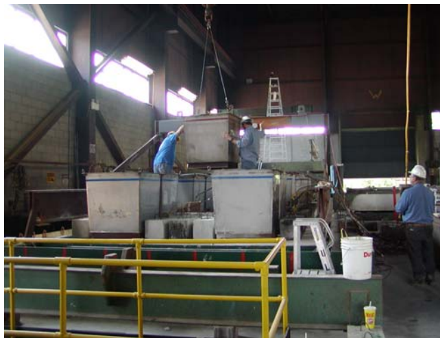
Figure 3–5. 35 ft span test assembly loaded with concrete blocks and water-filled containers.
