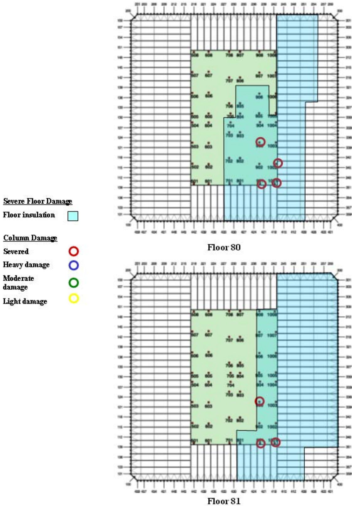
Figure B-14. WTC 2 Case C aircraft impact damage to Occupancy Floors 80 and 81.
