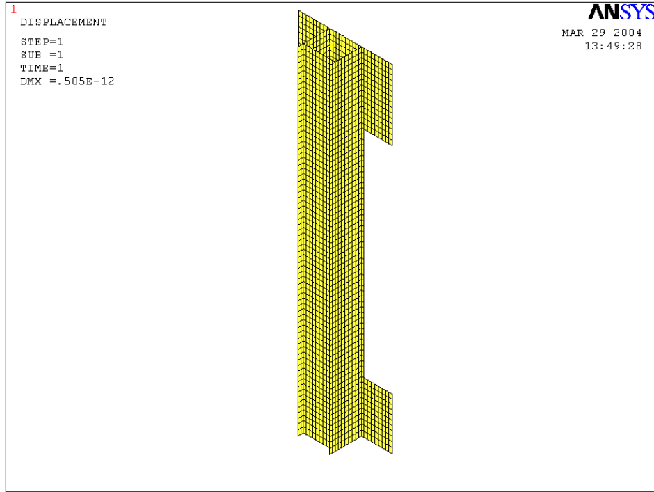
Figure 6-13. One-story exterior column model.
