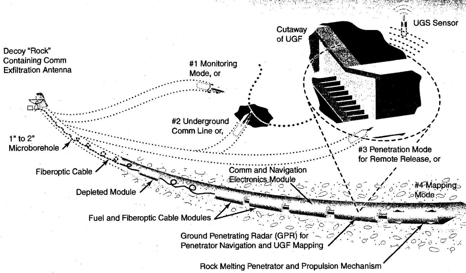
Figure 12. Original Phase I Proposal Configuration of the Proposed Rock-Melting Underground Microbore Showing Penetrator Tip, Navigating and Mapping Ground-Penetrating Radar Plus Sensors Module, a Communications and Underground Navigation Electronics Cylinder, and a Number Of Modules Containing Tip-Melting Fuel and Coiled Fiberoptical Comm Cable
