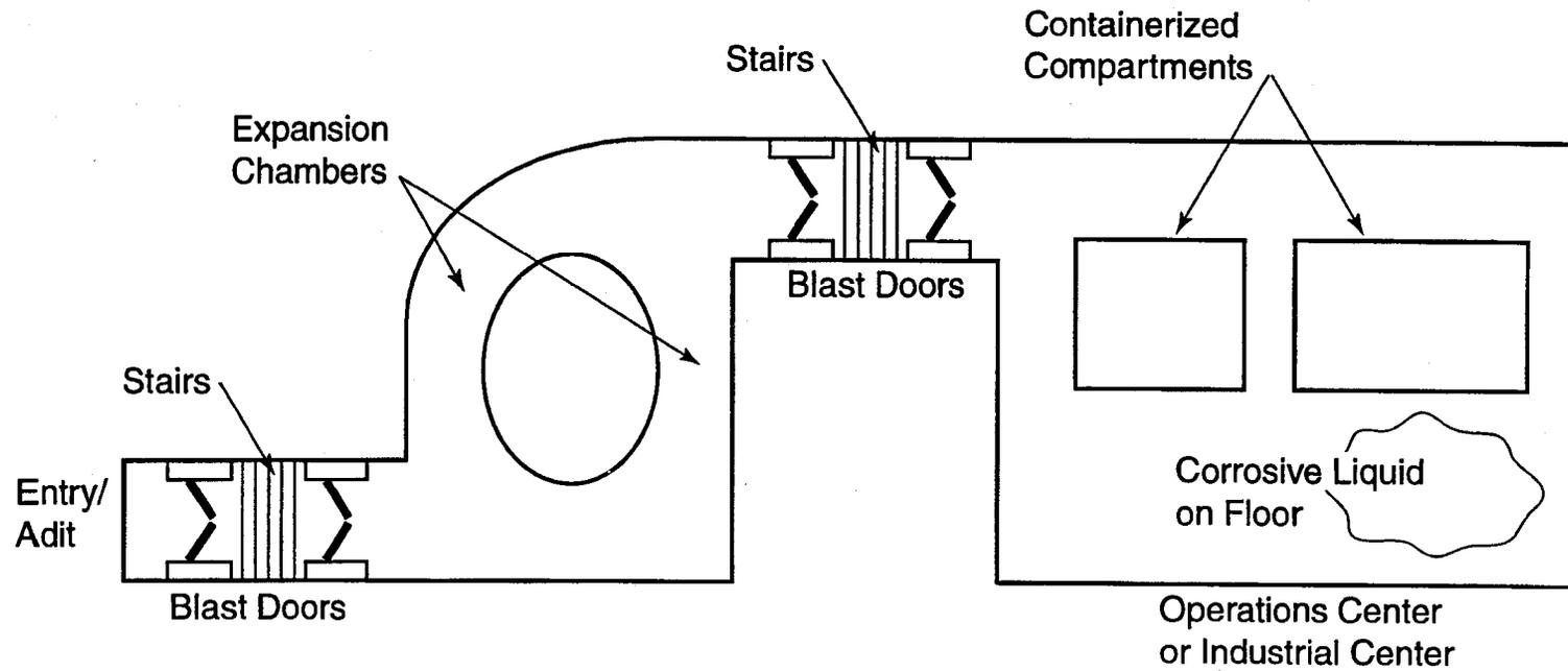
Figure 3. Prototypical Underground Facility System Layout, Overhead View
