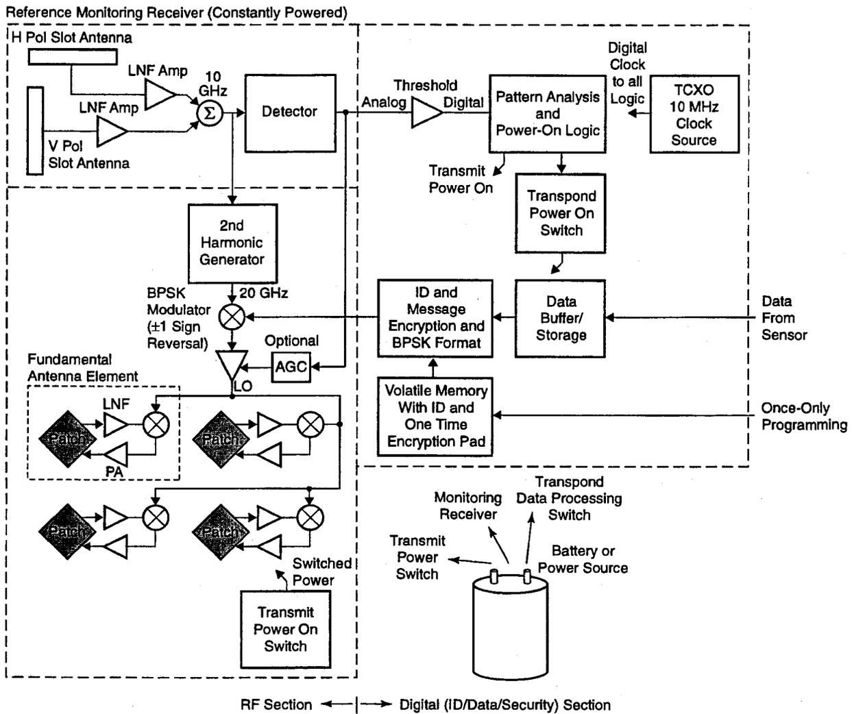
Figure 32. Architecture of Proposed Retrodirective Phased Array Data Exfiltration System
