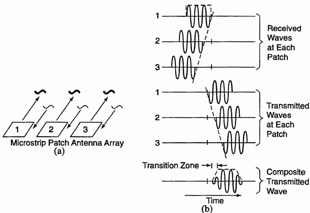
Figure 27. Illustration of the Transition Effect of Echoed Pulses From Retrodirective Phase Array Antennae. (a) Impinging wavefront on a linear array. (b) Time diagram of the phasing of the echoed pulse from the retrodirective array.
