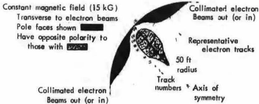
Fig. 8 — Space accelerator for SPEAR
