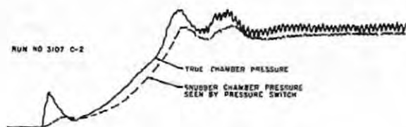
Figure 11. Gas Generator Start Transition (Typical P_c Trace Without Sequence Valve)
