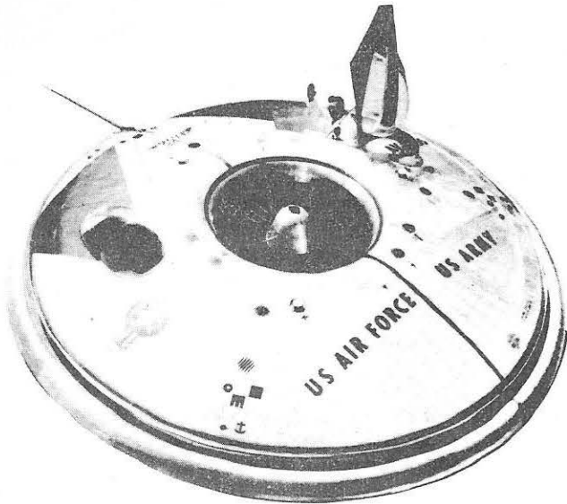
Disc-shaped AVROCAR, a research vehicle, was designed to explore potential of several new approaches to vertical takeoff and landing craft.
