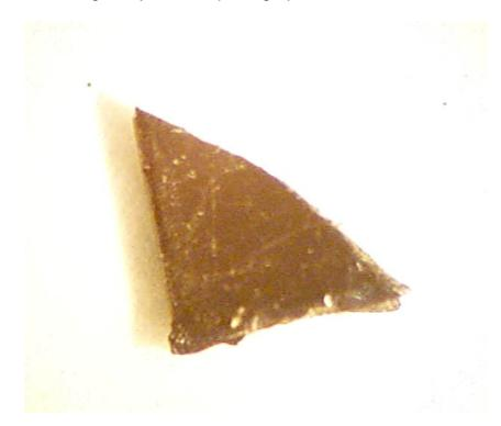
The infrared spectra taken from both sides of the object are identical. They identify the polymer as polycarbonate + poly(styrene:acrylonitrile:butadiene). These spectra match a reference of this material. Following are spectra from the sample and a reference of polycarbonate + poly(styrene:acrylonitrile:butadiene) for comparison.
