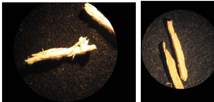
Reference photographs of splinters obtained from a 2X6 pine board (Left) and a twig (right)
