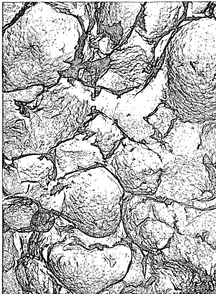
FIGURE 3.5 ELECTRON MICROSCOPE TRIAFOL REPLICA OF NON-IRRADIATED 20% U-235 O 2 - 80% ThO 2 (1150°C FIRED)
