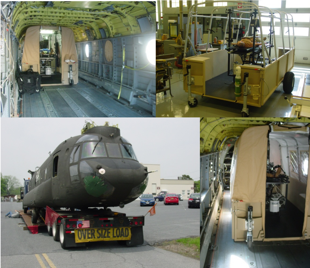
FIGURE 15: CH47 Roll-On/Roll-Off Treatment POD
