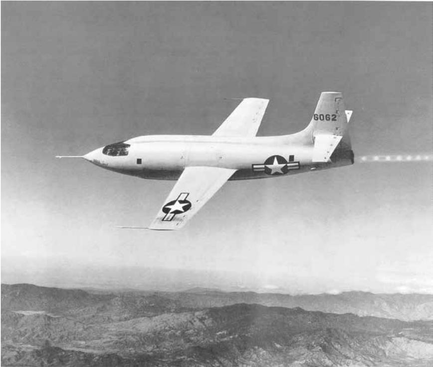
Bell XS-1 photographed on its way to becoming the first aircraft to exceed Mach 1 in level flight. (USAF)
