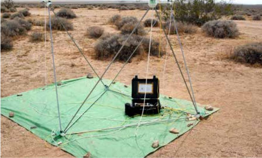
Boom Amplitude and Direction Sensor near Cords Road, August 2003. (NASA)
