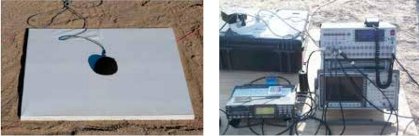
B&K microphone and recording equipment. (NASA)
