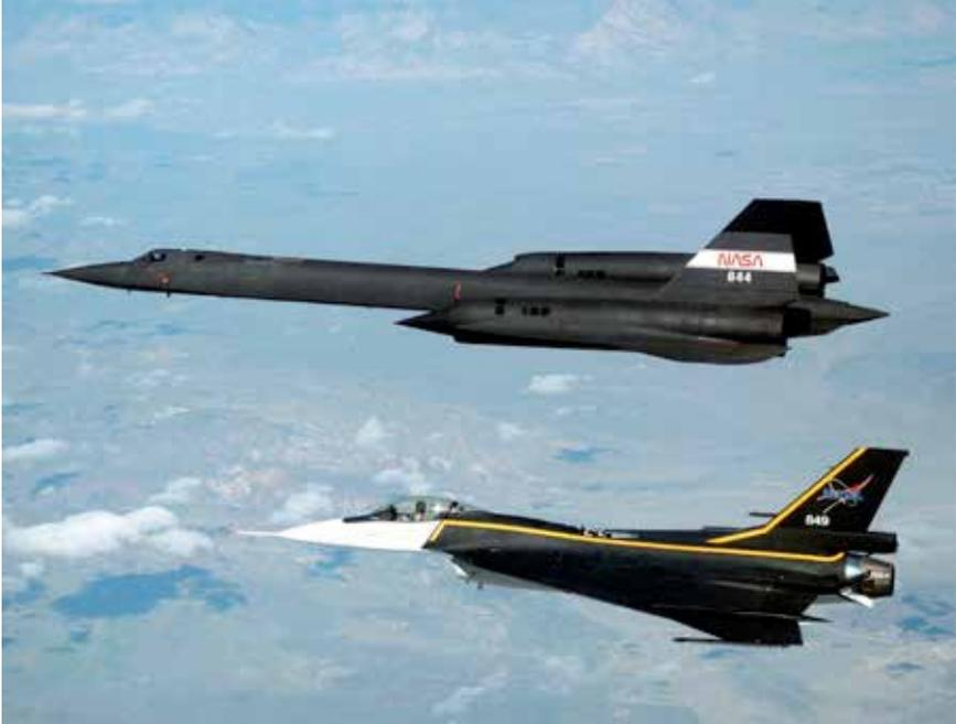
F-16XL and SR-71 during in-flight shock wave measurements in 1995. (NASA)
