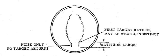
FIG. 4-24 APQ-56 MONITOR SCOPE TRACES - ALTITUDE SET LOW - AIRCRAFT WINGS LEVEL
