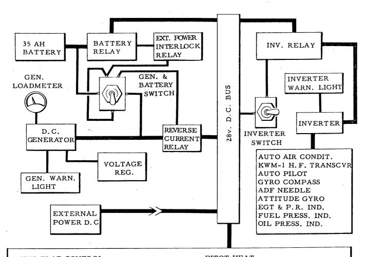
WING FLAP CONTROL LANDING GEAR CONTROL SPEED BRAKE CONTROL AILERON SHIFT ACTUATOR AILERON TRIM TAB ACTUATOR ELEVATOR TRIM TAB ACTUATOR WING FLAP POSITION INDICATOR LANDING GEAR POSITION INDICATOR LANDING GEAR WARNING FIRE WARNING WARNING LIGHTS COCKPIT LIGHTS LANDING LIGHTS ANTI-COLLISION LIGHTS FACE HEAT EMERGENCY FACE HEAT AIR CONDITIONING - MANUAL FUEL SHUT-OFF EMERGENCY FUEL CONTROL FUEL QUANTITY COUNTER **ENGINE START**
