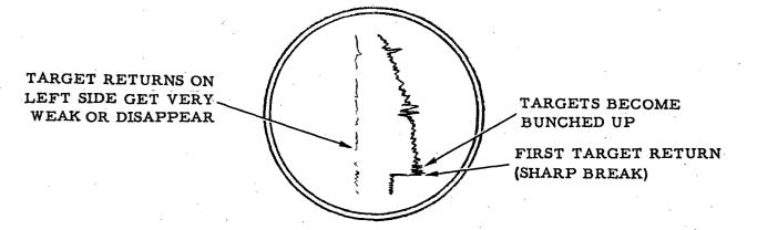
FIG. 4-25 APQ-56 MONITOR SCOPE TRACES ALTITUDE SET LOW - AIRCRAFT IN RIGHT BANK
