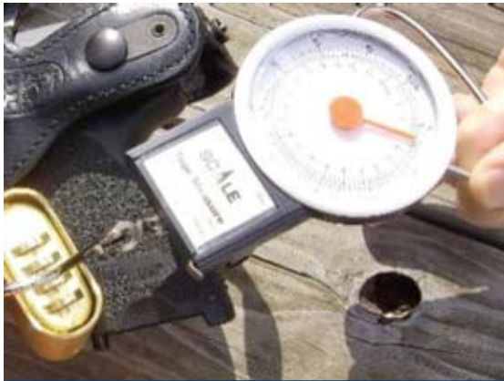
Measuring foot pounds of lateral force required to induce a weapon discharge.
