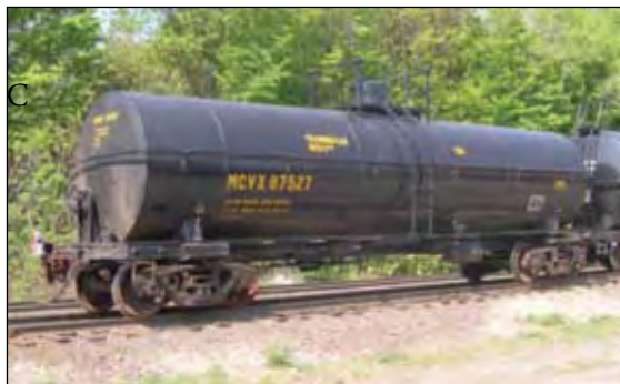
Chlorine Tank Car
