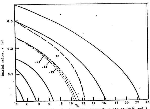
Evaporation of fine droplets into vapourfree air at 20 °C and 1 atm., with allowance for Kelvin effect and free molecular flow at surface (Ke=0.1). Initial radii 0.06, 0.12, 0.16, 0.30, 0.36  $\mu m$ , with allowance for Kelvin effect and free molecular flow at surface (Ke=0.04, 0.13, 0.19). Initial radius 0.24  $\mu m$ , with allowance for Kelvin effect alone. Diffusion control. Initial radius 0.30  $\mu m$ .
