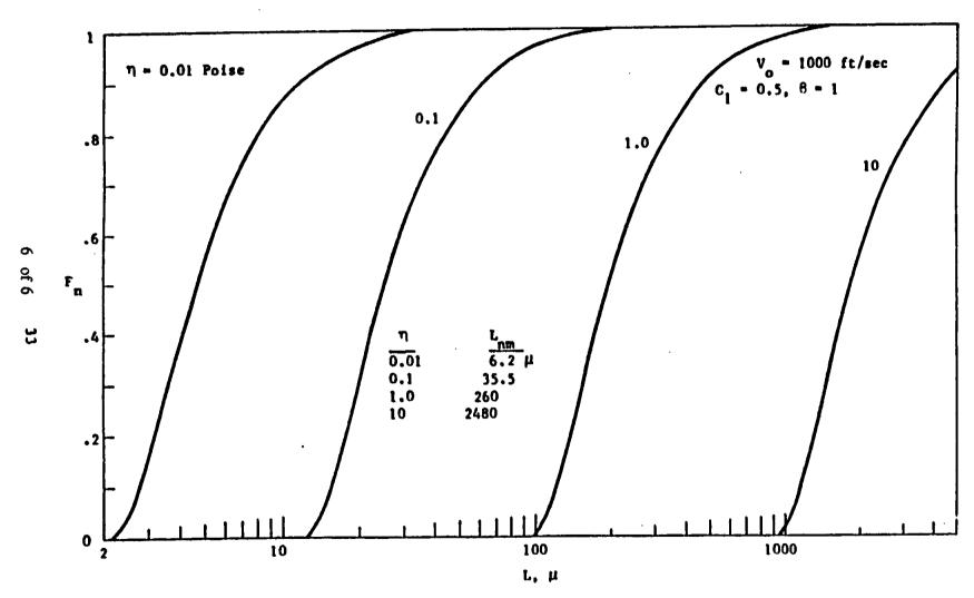
Figure 7. Effect of Fluid Viscosity on the Number Fraction Distribution.
