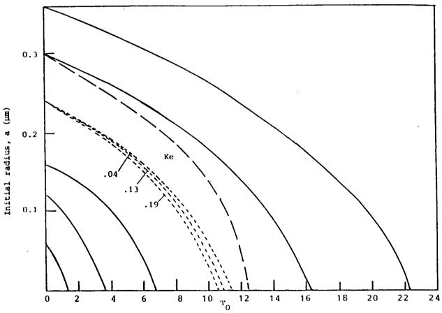
Figure 4.2 Evaporation of fine droplets into vapourfree air at 20 °C and 1 atm., with allowance for Kelvin effect and free molecular flow at surface (Ke=0.1). Initial radii 0.06, 0.12, 0.16, 0.30, 0.36  $\mu m$ , with allowance for Kelvin effect and free molecular flow at surface (Ke=0.04, 0.13, 0.19). Inital radius 0.24  $\mu m$ , with allowance for Kelvin effect alone. Diffusion control. Initial radius 0.30  $\mu m$ .
