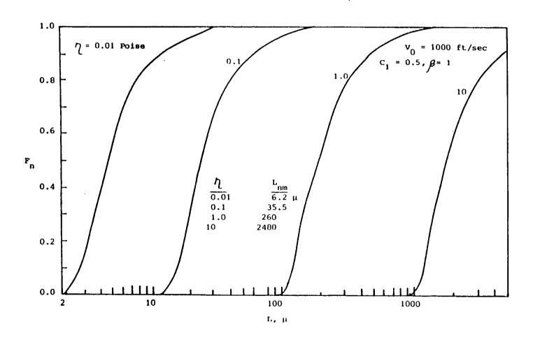
Figure 4.4 Effect of Fluid Viscosity on the Number Fraction Distribution
