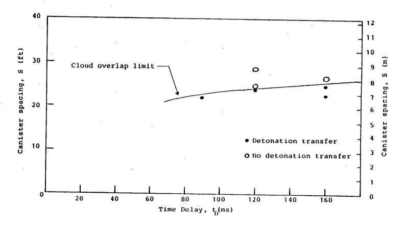
Figure 5.3 Results of detonation transfer experiments. Spacing, S, between canisters versus delay time,  $t_{\rm c}$  between burster initiation and cloud detonation. Propylene oxide fuel, 2 gallons, 1/d = 2, F/B = 90.
