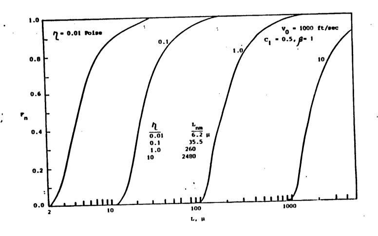
As discussed previously, the primary stripping breakup of a liquid produces a spectrum of particles (drops) whose sizes range from the minimum size, which is determined by wind velocity and fluid viscosity, to the maximum size which is proportional to the linear dimensions of the liquid. A portion of these drops then continue to uncergo secondary (and higher order) breakup during their drag deceleration to a stable size.
