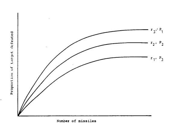
Figure 8.4 Proportion of target defeated as a function of the number of missiles delivered
