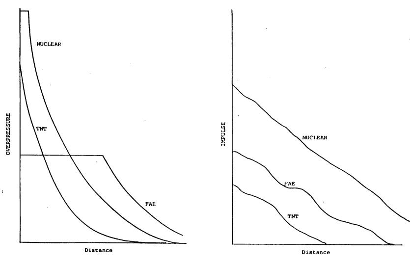
Figure 6.1 Qualitative comparison of blast parameters of convential, nuclear and FAE explosives of similar yield
