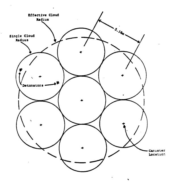
Figure 5.4 Sketch showing the relative positioning of the individual canisters. The seven circles represent the FAE clouds from the
