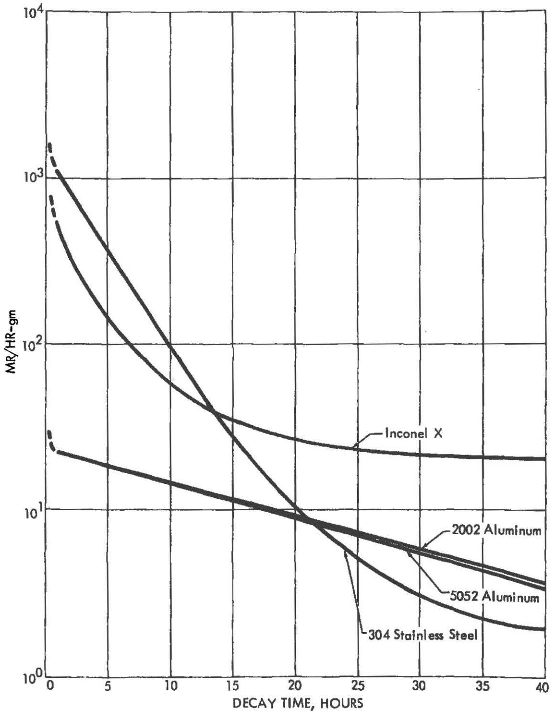
FIGURE 30 INDUCED GAMMA ACTIVITY IN CRYOSTAT (SHIELDED)
