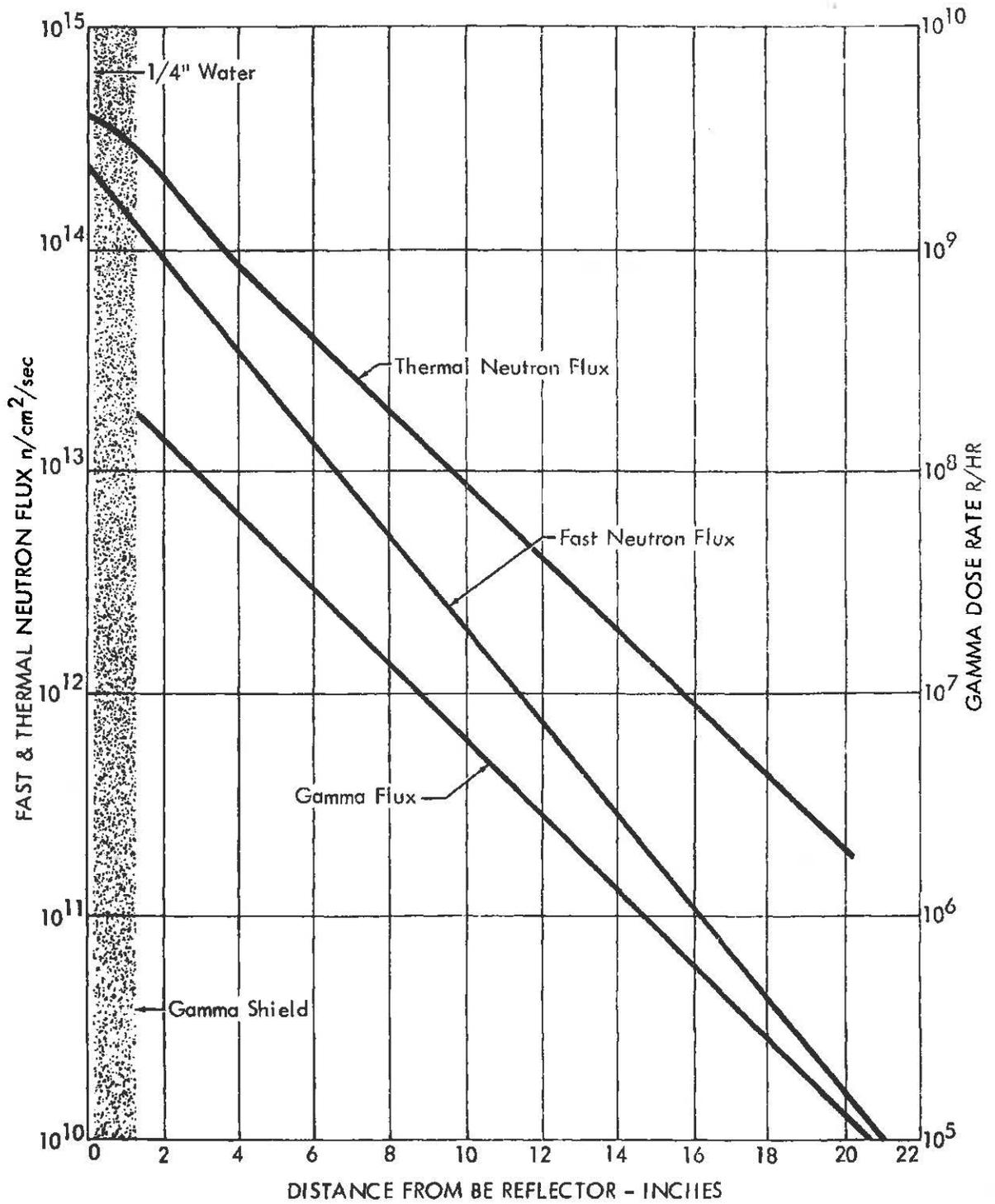
FIGURE 24 AXIAL FAST NEUTRON FLUX, THERMAL NEUTRON FLUX AND GAMMA FLUX IN HB-2 TUBE FROM BE REFLECTOR FACE WITH GAMMA SHIELD
