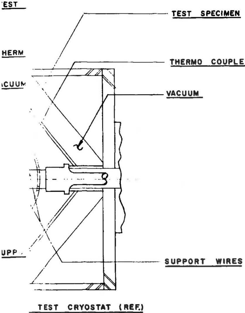
**TEST CRYOSTAT (REF.)**
