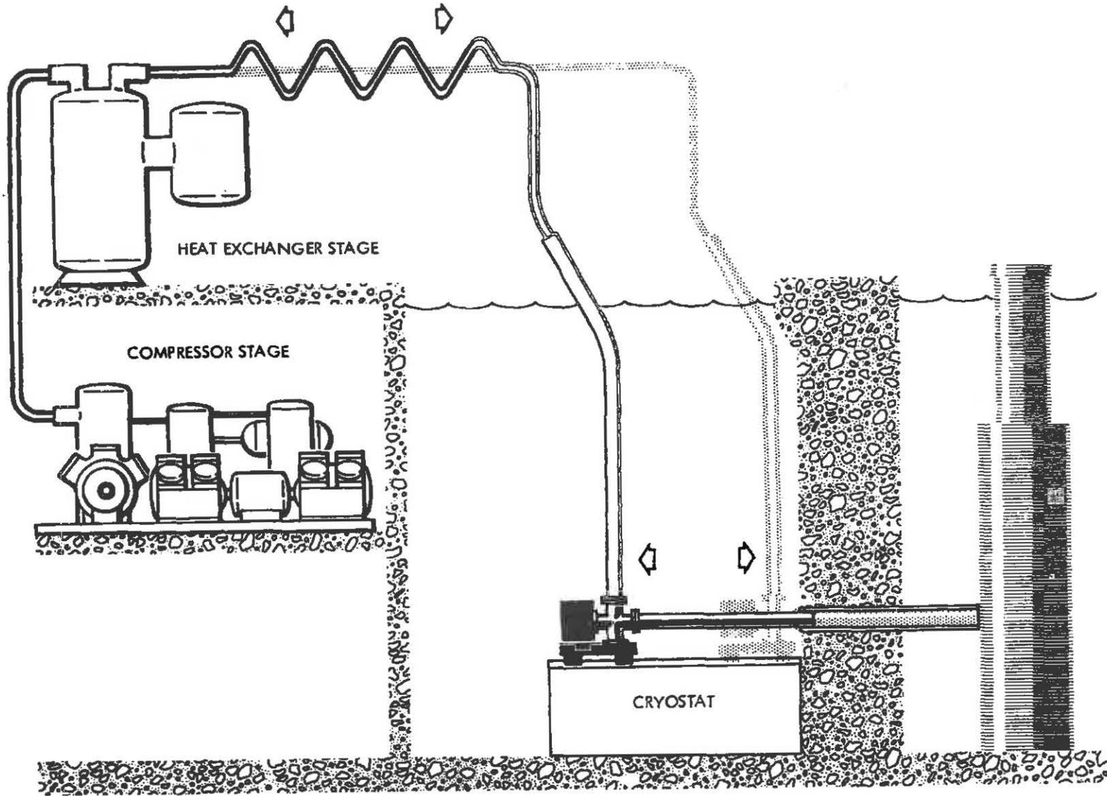
FIGURE 17 CRYOSTAT HORIZONTAL MOVEMENT SCHEMATIC
