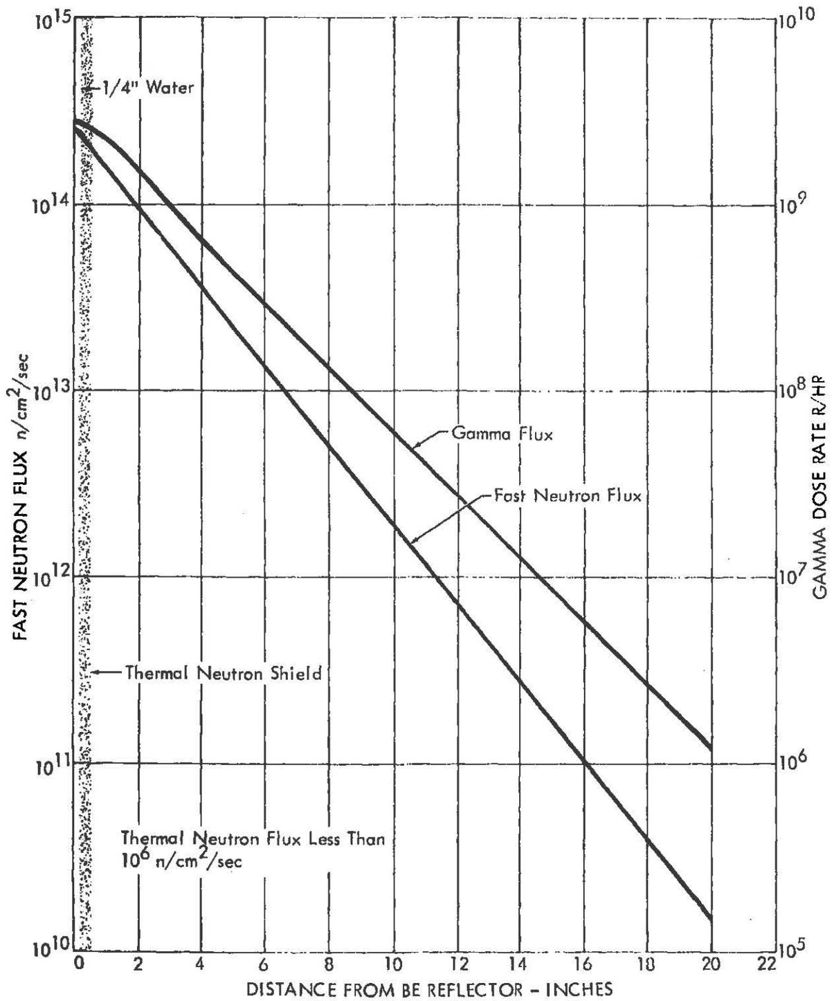
FIGURE 25 AXIAL FAST NEUTRON FLUX, GAMMA FLUX IN HB-2 TUBE FROM BE REFLECTOR FACE WITH THERMAL NEUTRON SHIELD
