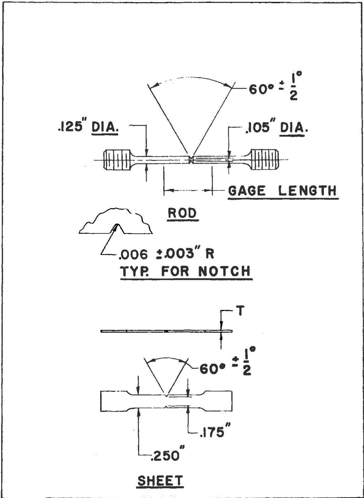
FIGURE 5 TENSILE TEST SPECIMENS - NOTCH SENSITIVITY
