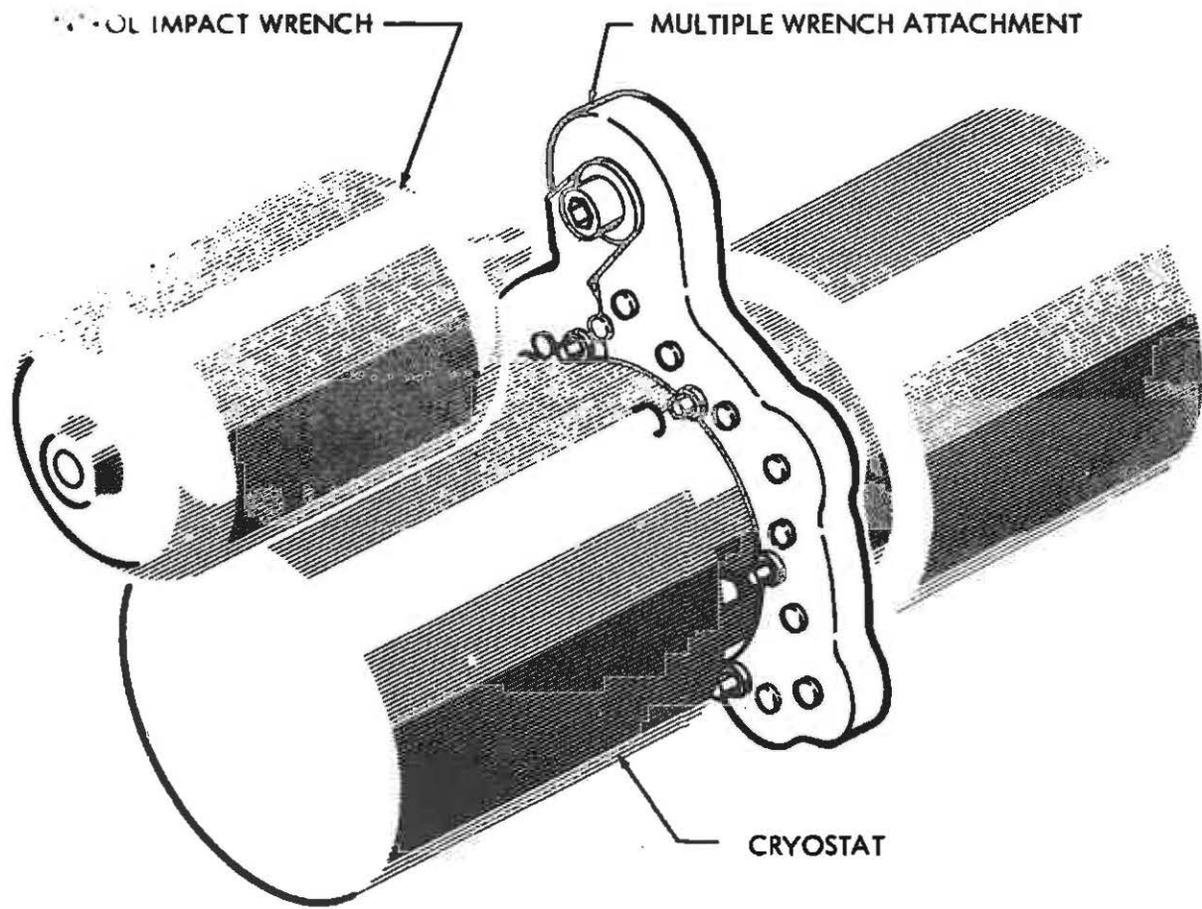
FIGURE 19 CRYOSTAT REMOVAL WRENCH ASSEMBLY - BACK FLANGE
