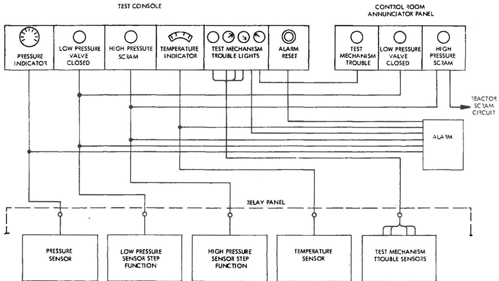
FIGURE 28 ALARM SYSTEM SCHEMATIC
