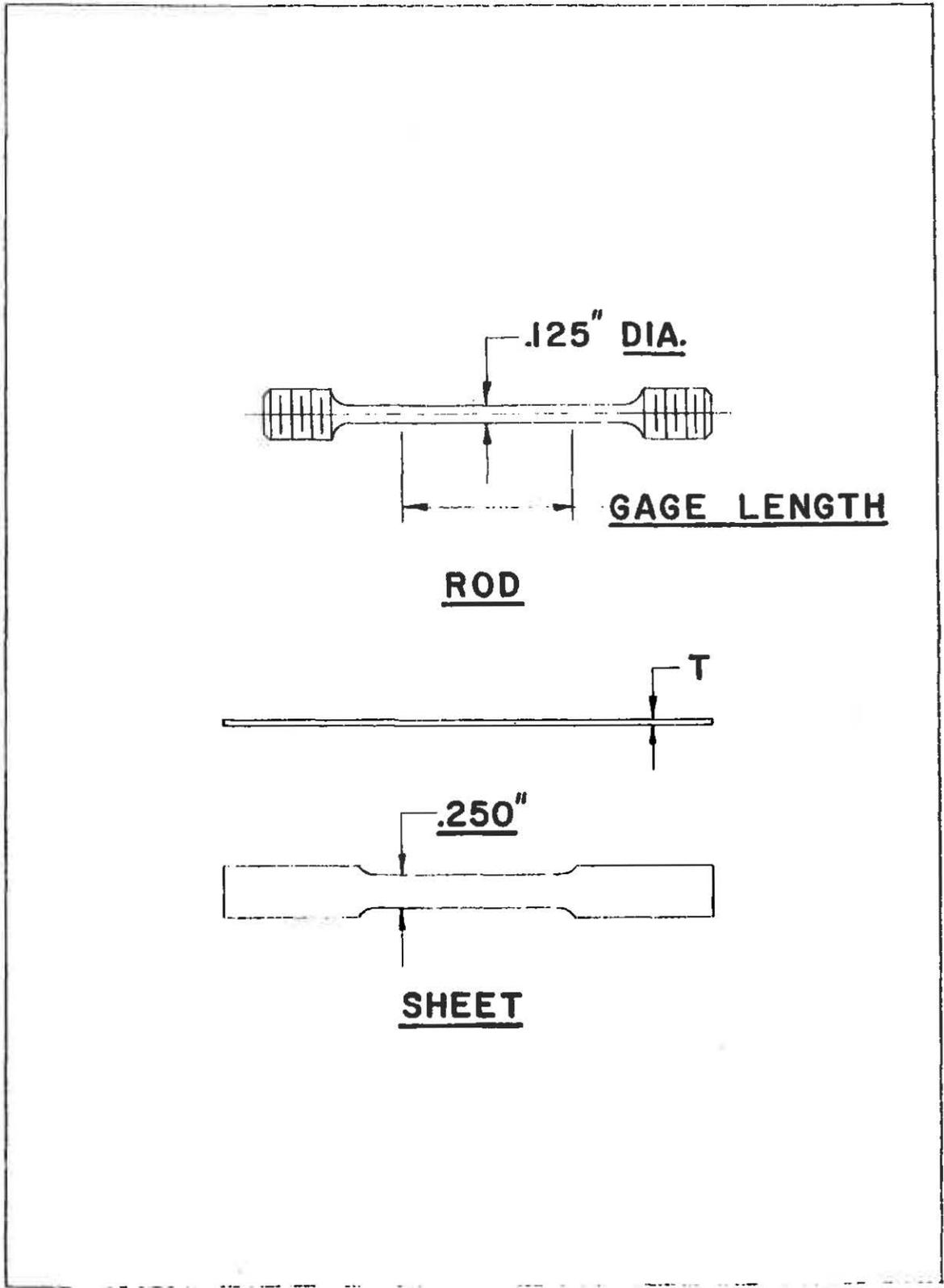
FIGURE 8 CREEP TEST SPECIMENS
