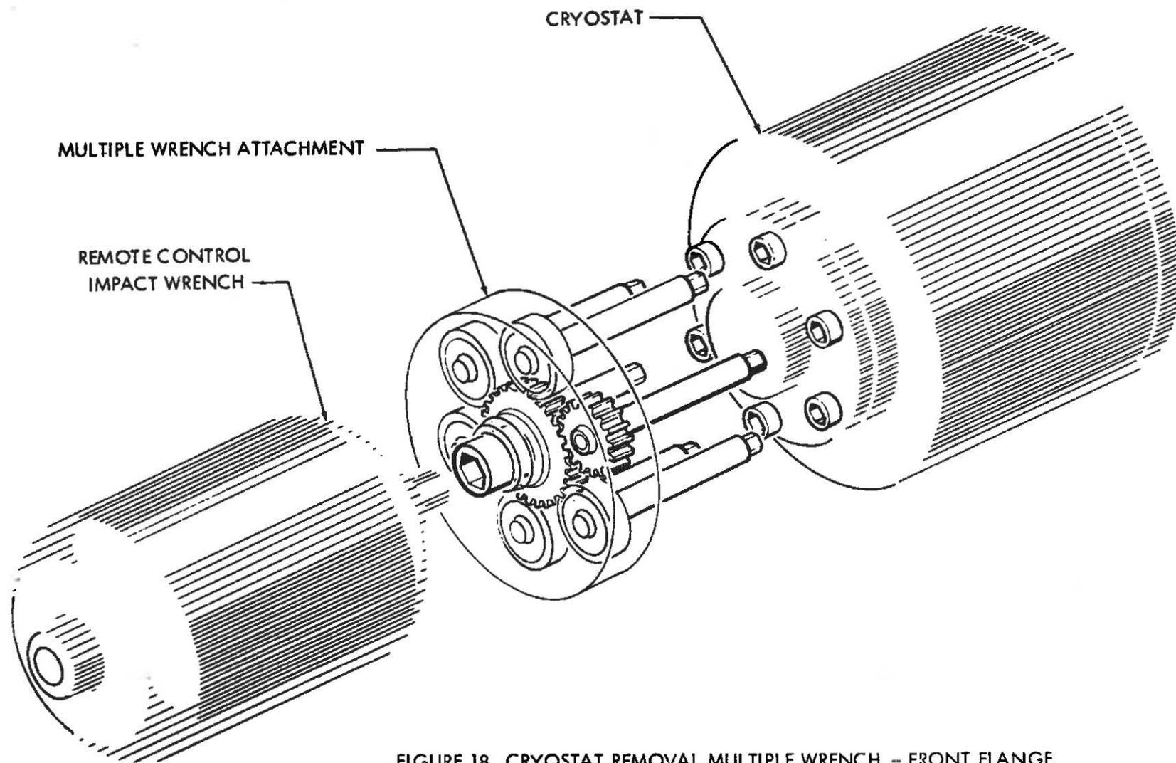
FIGURE 18 CRYOSTAT REMOVAL MULTIPLE WRENCH - FRONT FLANGE
