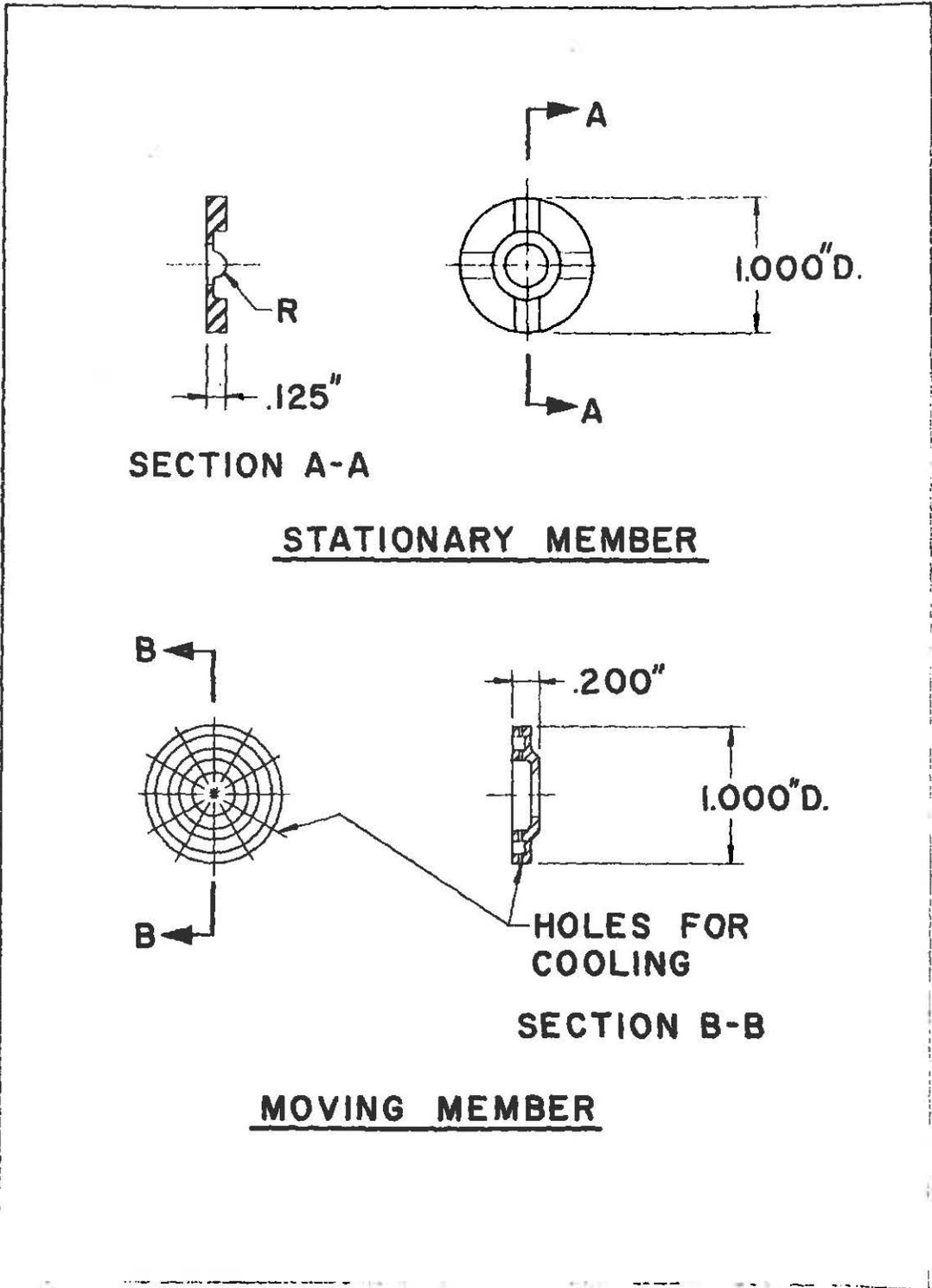
FIGURE 10 WEAR TEST SPECIMEN
