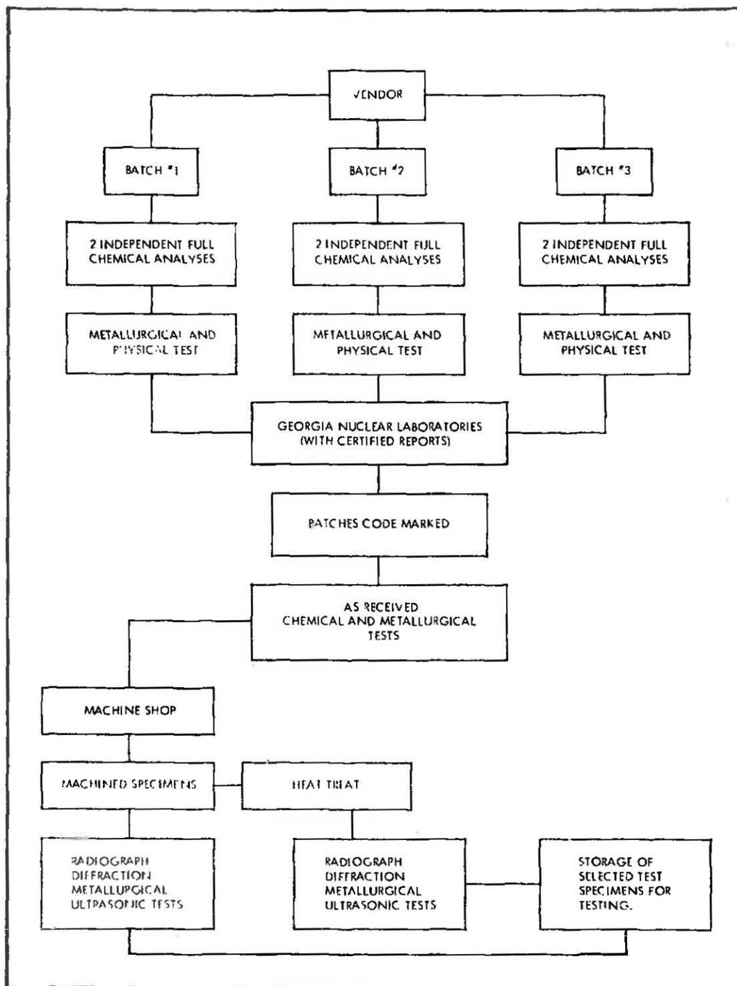
FIGURE 20 SPECIMEN PREPARATION FLOW DIAGRAM
