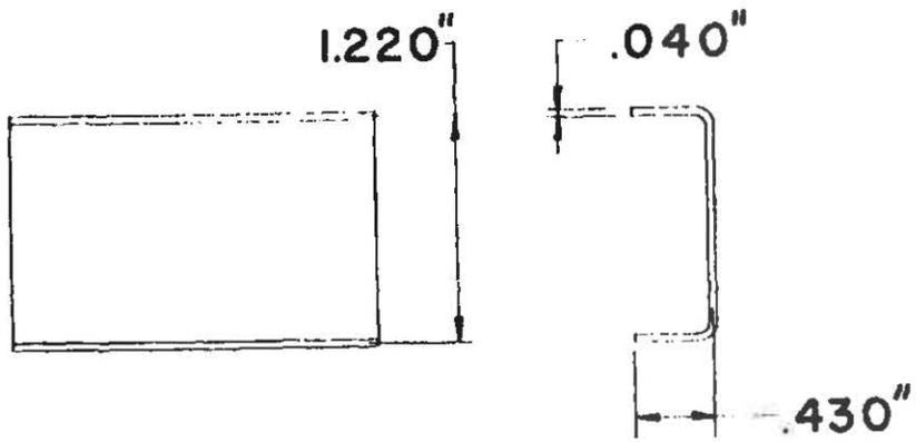
FIGURE 7 BUCKLING TEST SPECIMEN
