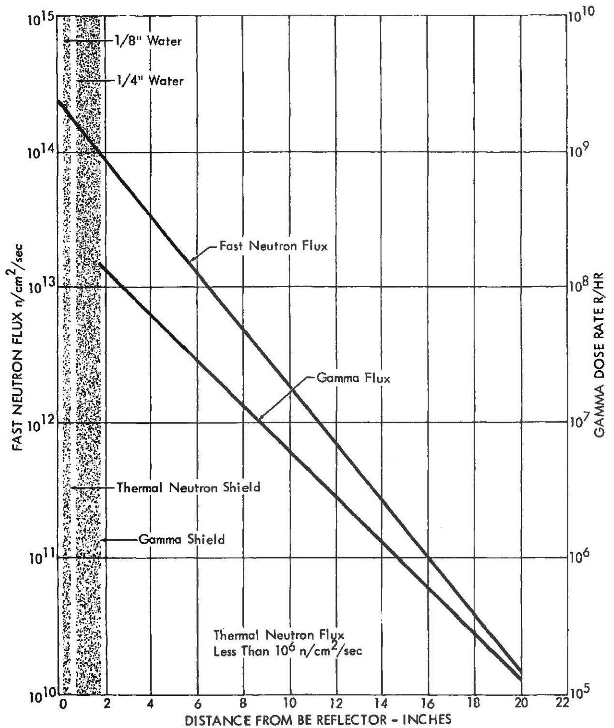
FIGURE 26 AXIAL FAST NEUTRON FLUX, GAMMA FLUX IN HB-2 TUBE FROM BE REFLECTOR FACE WITH THERMAL NEUTRON AND GAMMA SHIELDS
