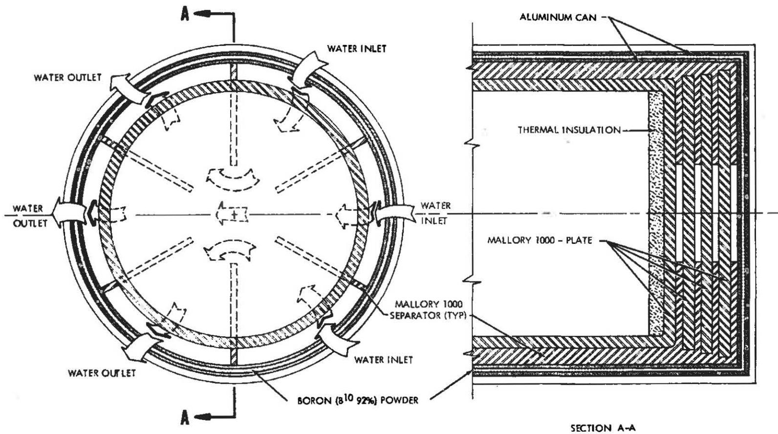
FIGURE 27 SHIELD TUBE COOLING
