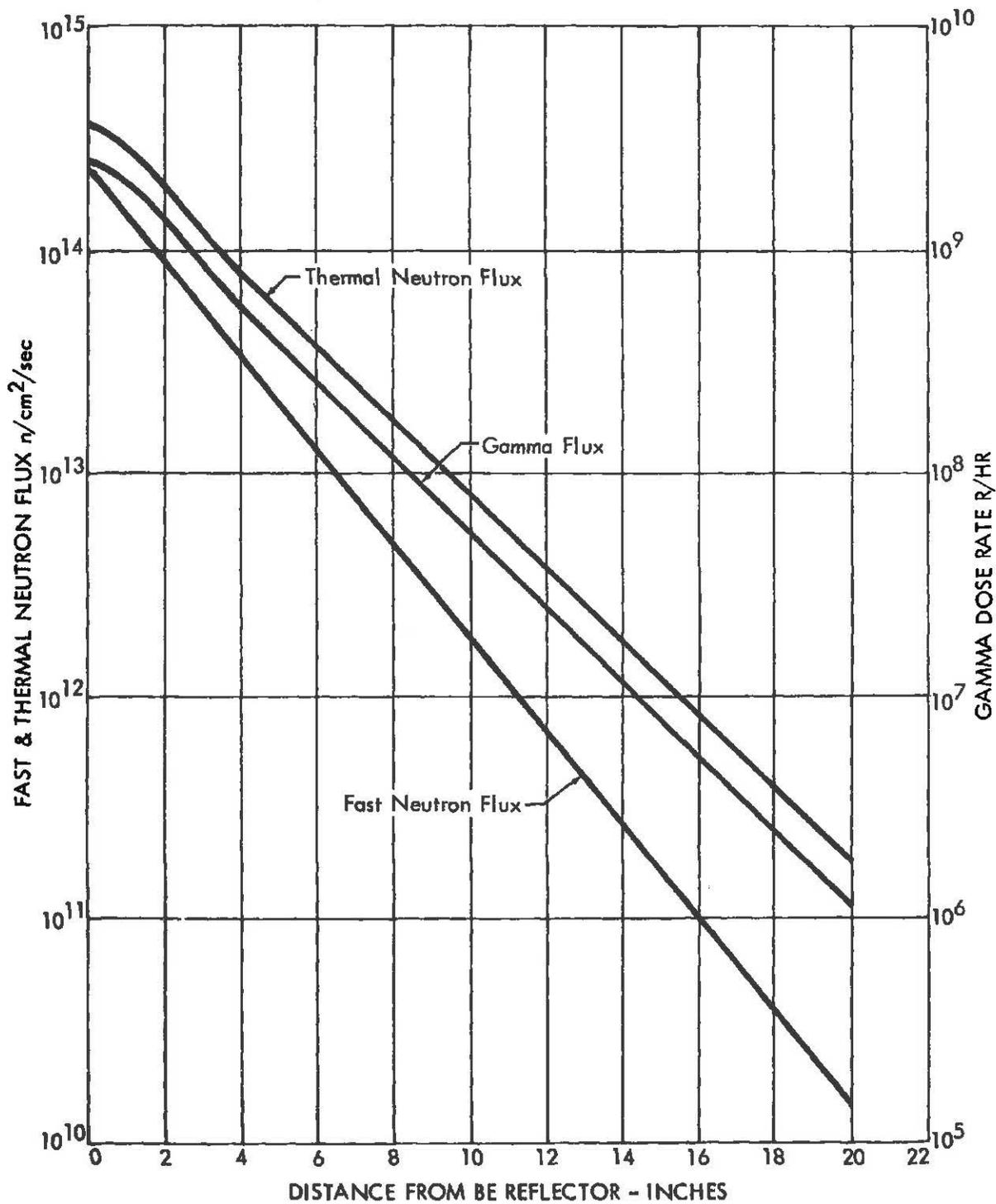
FIGURE 23 AXIAL FAST NEUTRON FLUX, THERMAL NEUTRON FLUX AND GAMMA FLUX IN HB-2 TUBE FROM BE REFLECTOR FACE
