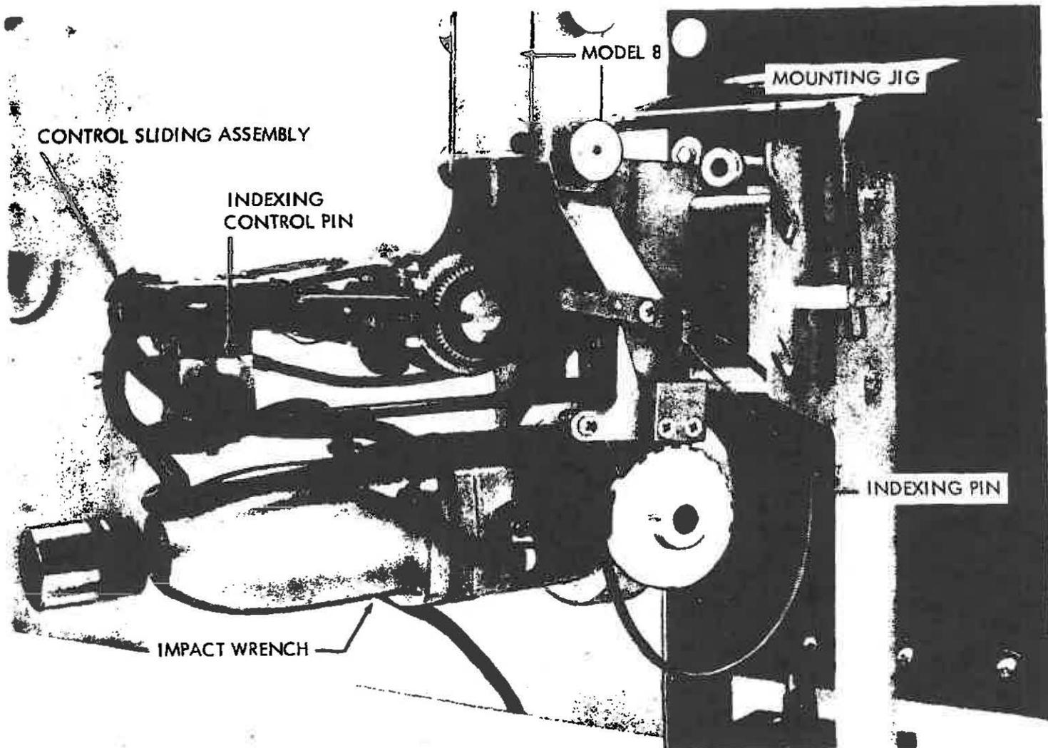
FIGURE A-2 IMPACT WRENCH BEING MOUNTED ON MODEL-8 MANIPULATOR
