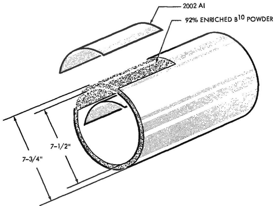
FIGURE 29 THERMAL NEUTRON SHIELD
