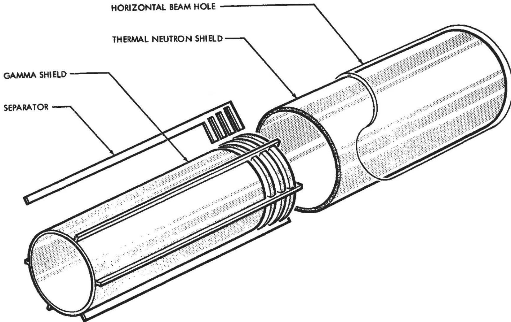
FIGURE 22 SHIELDING CONFIGURATION, EXPLODED VIEW
