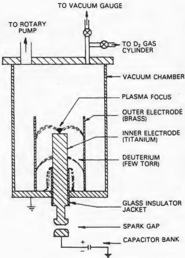
Fig. 1. Schematic of a plasma focus device.
