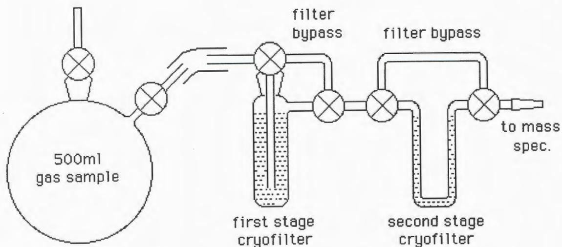
**Liquid Nitrogen cooled two stage activated charcoal cryofilter removes  $D_2$  and  $O_2$  from gas sample.**
