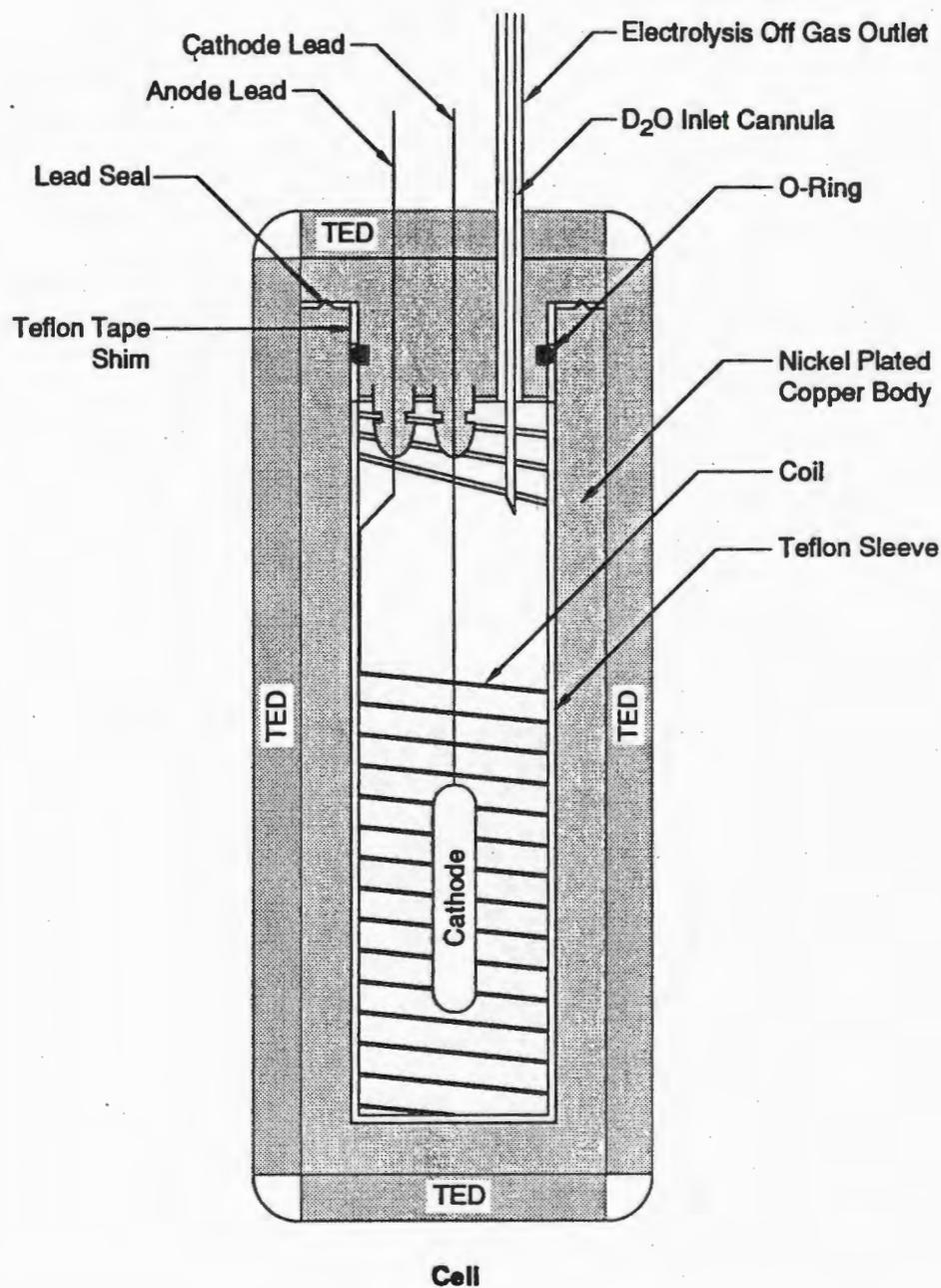
**All Metal cell, using metal seals throughout system. Helium can not diffuse through seals.**
