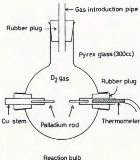
Fig. 1. Schematic diagram of the reaction bulb.
