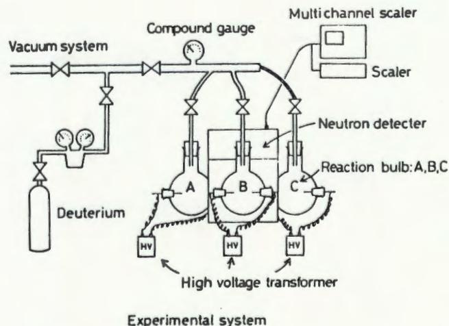
Fig. 2. Schematic diagram of the neutron measuring system.
