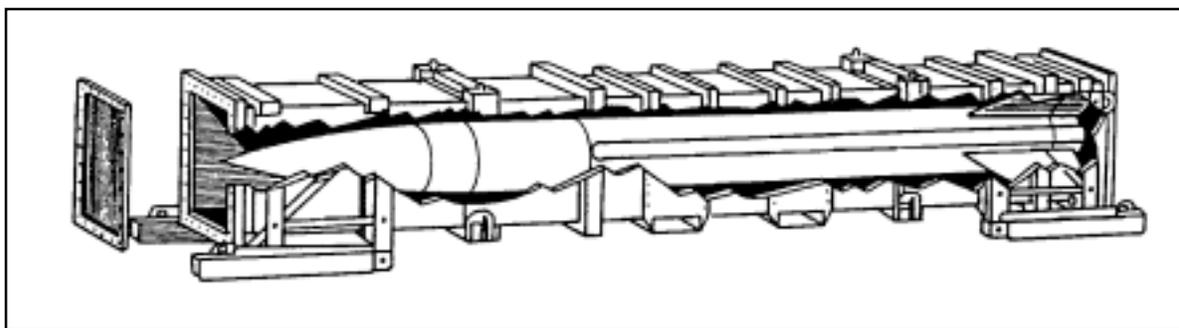
**Figure 5-7. Missile Canister**
