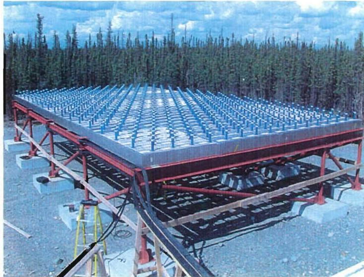
Figure B2. HAARP installation of the 16-panel AMISR prototype antenna.
