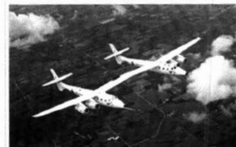
(U) Virgin Galactic WhiteKnightTwo is designed to reach an altitude of 50,000 feet (15.5 km) and release SpaceShipTwo, which will transport passengers to space at 361,00 feet (110 km) in the future. Courtesy Reuters
