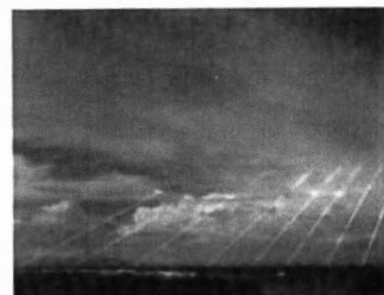
Testing at the Kwajalein Atoll of the Peacekeeper re-entry vehicles, all eight fired from only one missile. Each line, were its warhead live, represents the potential explosive power of about 375 kilotons.
