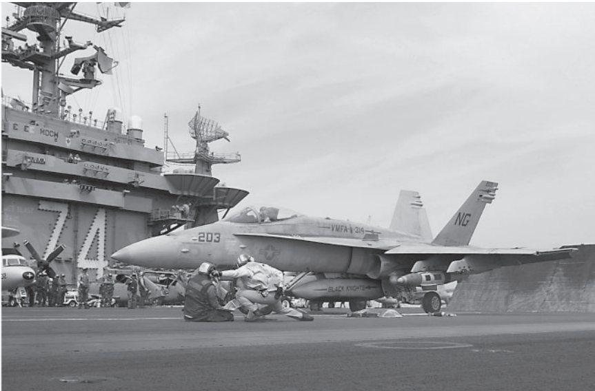
Cocked and ready. This F/A-18C armed with GBU-31 JDAMs and attached to Marine Fighter/Attack Squadron 314 aboard the aircraft carrier USS John C. Stennis is poised on the catapult moments before being launched on a mission into Afghanistan that could last as long as eight hours. Marine Corps strike fighter aviation is now almost fully integrated into the Navy's 10 carrier air wings.
