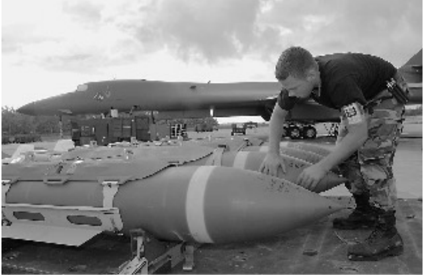
Trouble for the Taliban. A munitions technician prepares a pallet of 2000-lb GBU-31 satellite-aided JDAMs for loading into one of the bomb bays of this B-1B bomber operating against Taliban and al Qaeda targets out of Diego Garcia in the Indian Ocean. Over the course of Operation Enduring Freedom, B-1Bs dropped more than twice as many JDAMs as all other U.S. combat aircraft combined.
