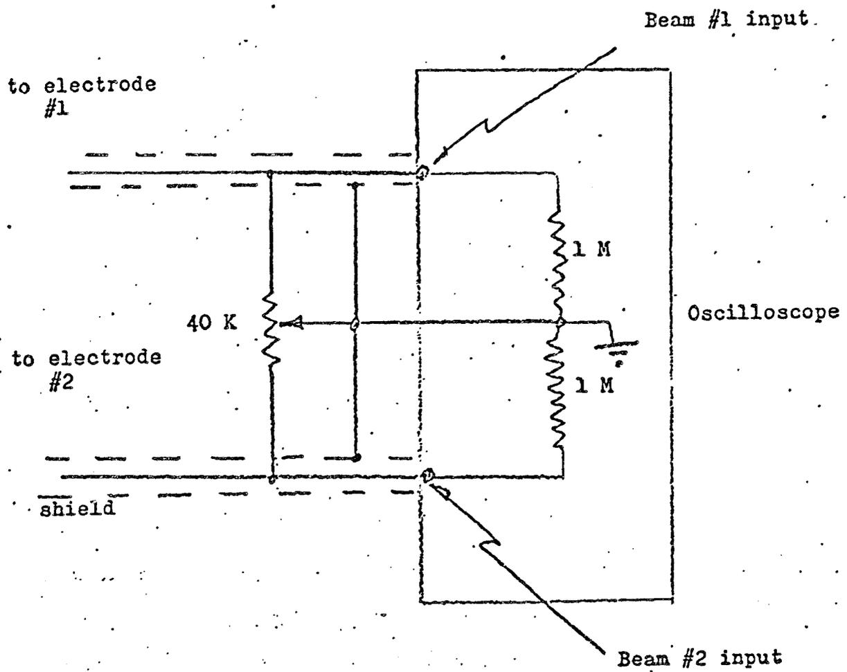
Figure 6. Input impedance reduction network.
