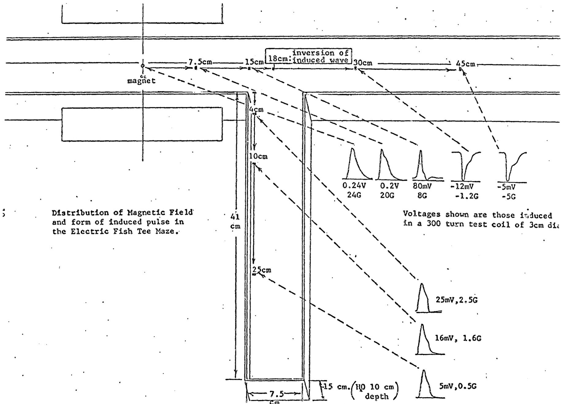
Distribution of Magnetic Field and form of induced pulse in the Electric Fish Tee Maze.
