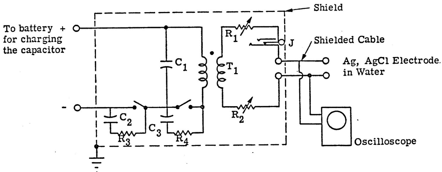
$C_1$  = High capacity tantalitic capacitor (value to be experimentally established according to the impedance of the electrodes in the water)
