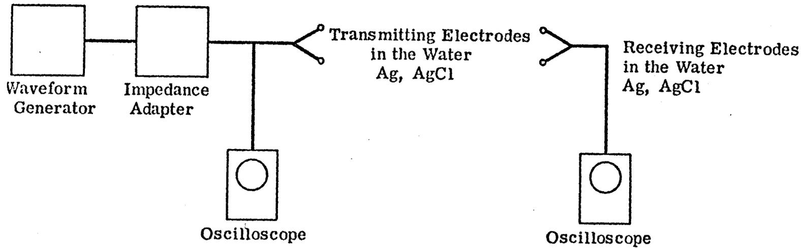
Fig. 7. Set-up for sinusoidal AC and square waves.
