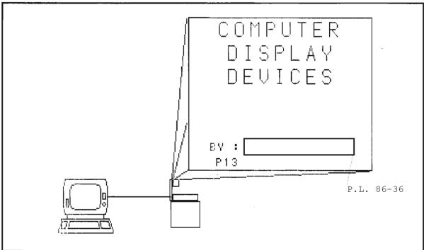
If you have to brief a number of people about some new software, you need to use a data display device, for no more than two people can read what's on a PC monitor at the same time. The device is attached to the computer and projects a screen image onto the wall using an overhead projector.
