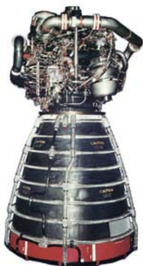
Figure 6-84. RS-25 (Altitude-Start SSME)
